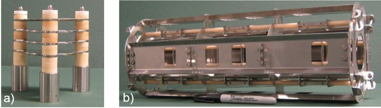
Figure 3.11: a) Four ring LAS extraction system used to accelerate ions to 5 keV beam energy. b) Electrostatic quadrupole triplet for additional focusing before the 90 degree bend to the main LEBIT beamline.
