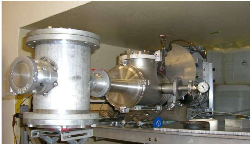
Figure 4.25: The PSSD mounted past the ISO160 tee, at the eventual location of the beam window of the prototype AT-TPC.
