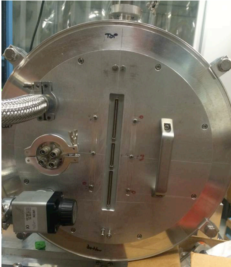
Figure 4.10: Image of the downstream ISO 400 flange. Readout electronics for the Micromegas are mounted on the vertical feedthroughs on the center of the flange. On the left of the flange, there are the both a gas inlet and outlet, as well as a KF40 flange with four SHV feedthroughs.
