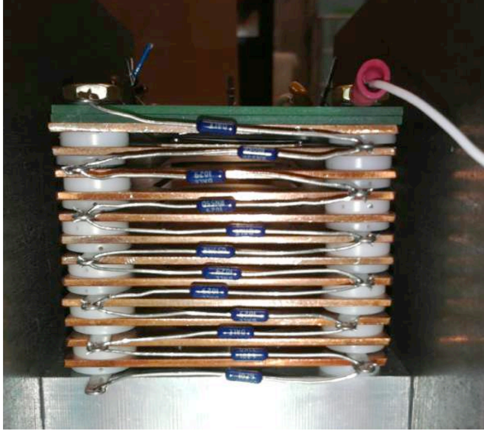
Figure 4.21: A side view of the copper plates and resistor chain on the MCP housing. The MCP and foil are both located on the green PCB on the top of the chain.
