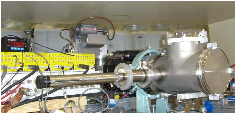
Figure 4.20: Image of the ISO160 tee with the retracting beam ladder. The MCP is mounted on the top flange and is install inside of the tee. The black beam steerer can be seen located a few inches upstream of the tee.
