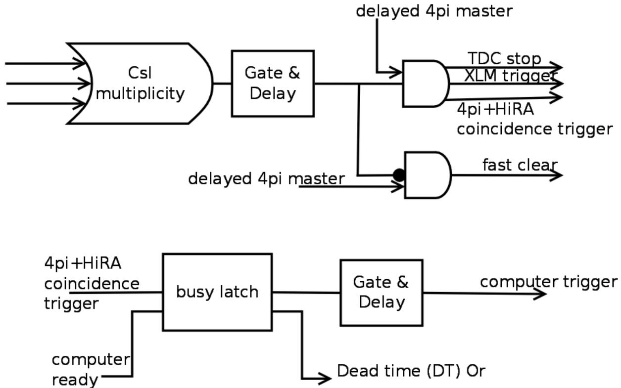
Figure 2.18: Diagram of the coincidence trigger logic. [6]
