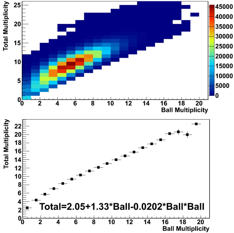
Figure 3.24: The relationship between the total multiplicity in the  $4\pi$  array and the multiplicity in the ball elements of the array is shown in the upper panel. The lower panel shows the mean total multiplicity as a function of ball multiplicity.
