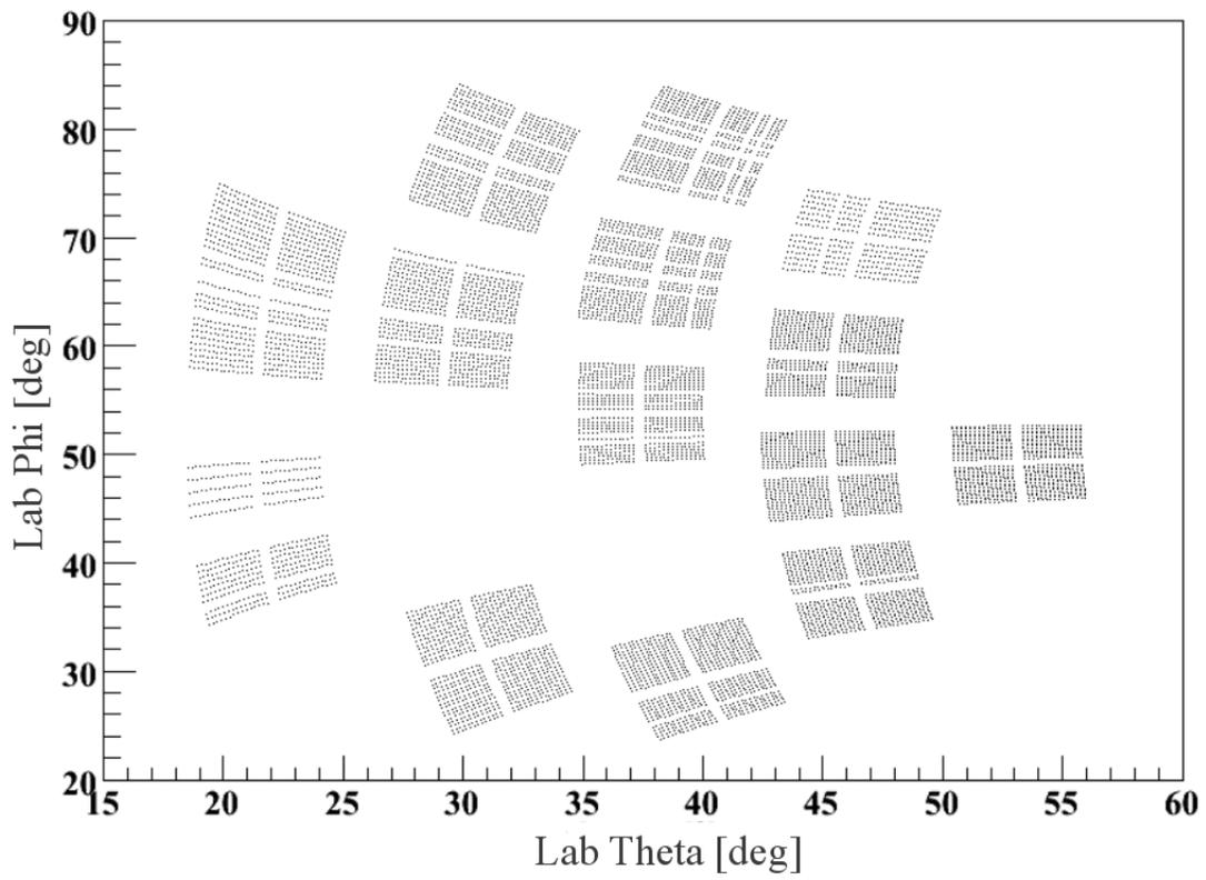
Figure 2.8: Actual angular coverage of the HiRA array.
