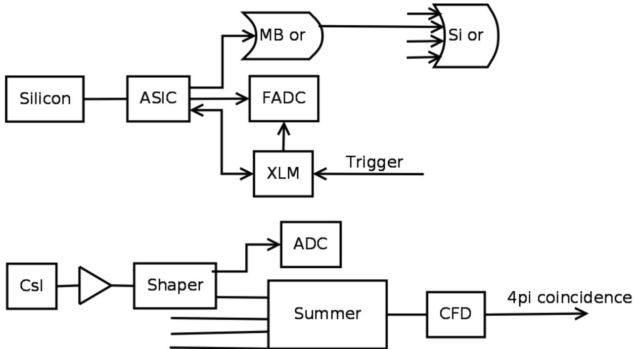
Figure 2.14: Diagram of the HiRA electronics logic. [2, 4]
