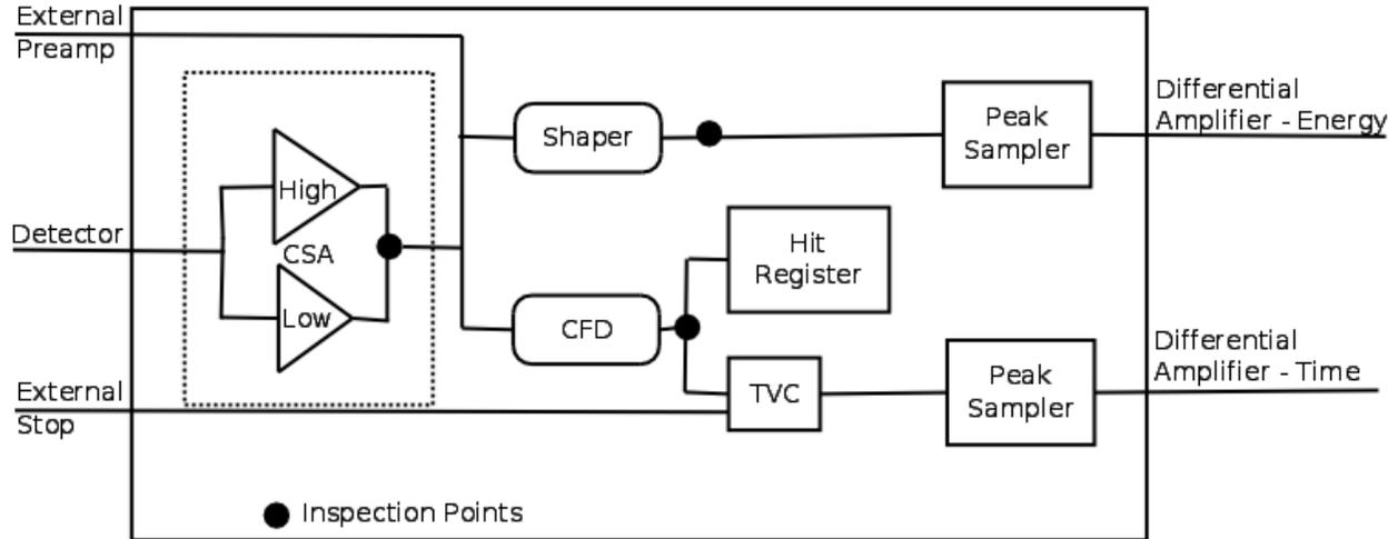
Figure 2.13: Diagram of the ASIC electronics logic. [2,3]
