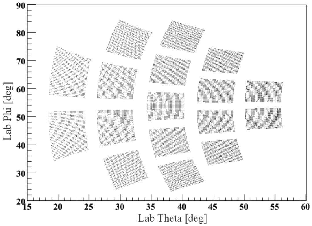
Figure 2.7: Angular coverage of the entire HiRA array.
