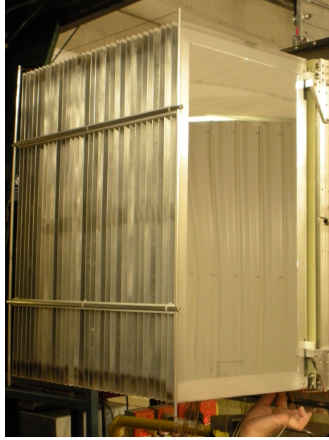
Figure 2.5: Photograph of the alternating cathode and anode plates of the ionization chamber. Plates are oriented perpendicular to the beam axis.
