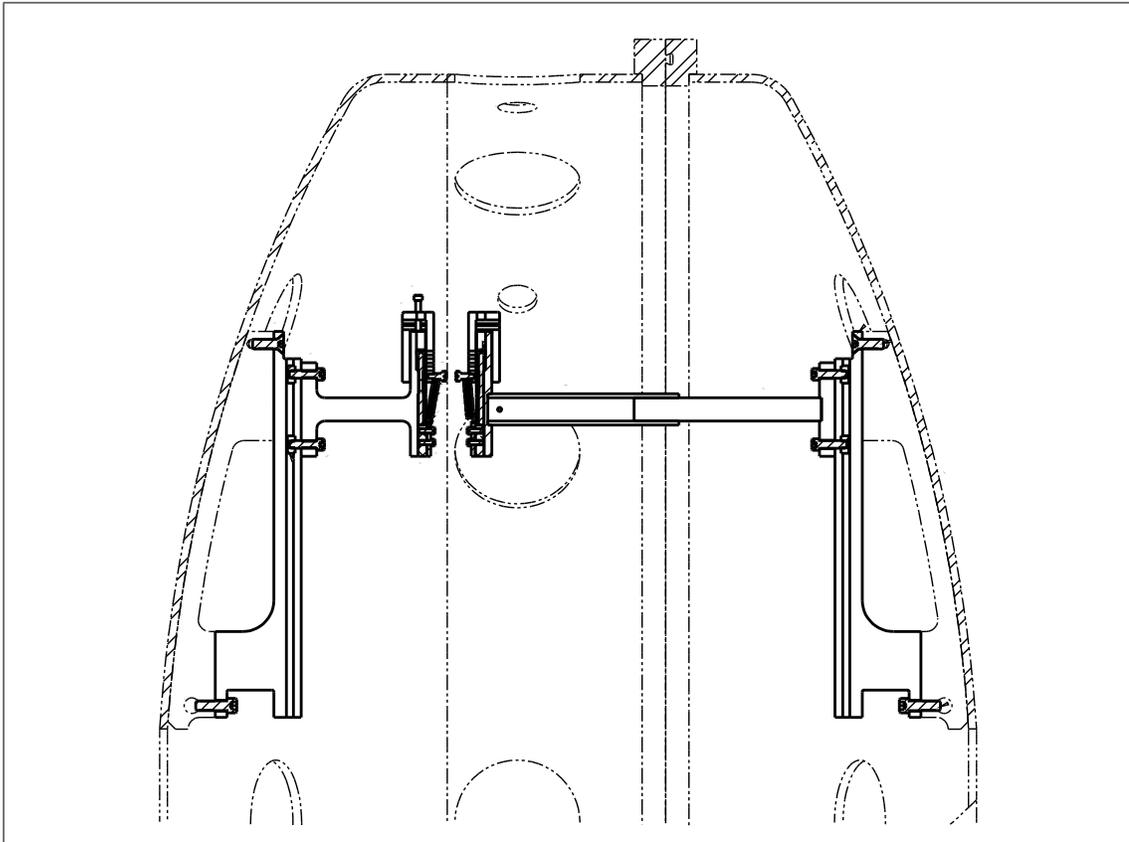
Figure 3.2. Mechanical drawing of the rf carpet test stand and the original carpet and push electrode supports. The (dot-dot-dash) lines show the rf carpet test stand and the (solid) lines show the carpet and push electrode supports.
