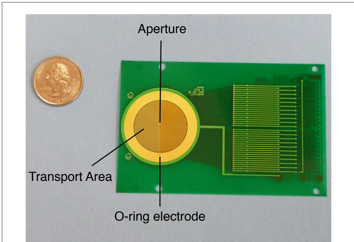
Figure 3.46. Photograph of the extraction rf carpet from Wada [5] with an aperture used for ion extraction measurements. The outer o-ring electrode was used to confine the ions on the rf carpet.
