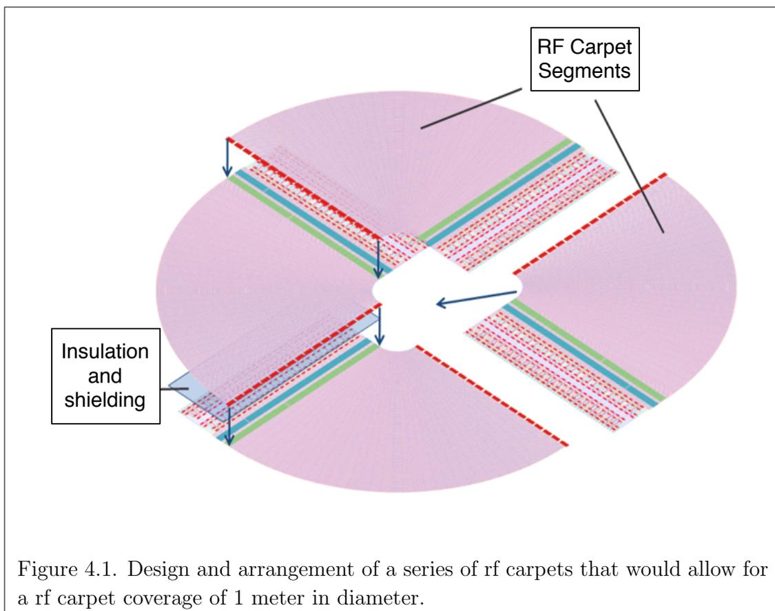
Figure 4.1. Design and arrangement of a series of rf carpets that would allow for a rf carpet coverage of 1 meter in diameter.
