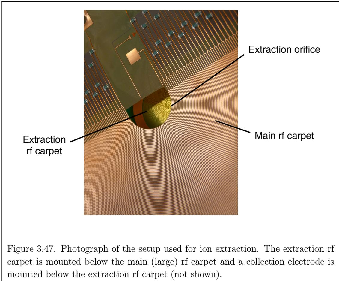
Figure 3.47. Photograph of the setup used for ion extraction. The extraction rf carpet is mounted below the main (large) rf carpet and a collection electrode is mounted below the extraction rf carpet (not shown).
