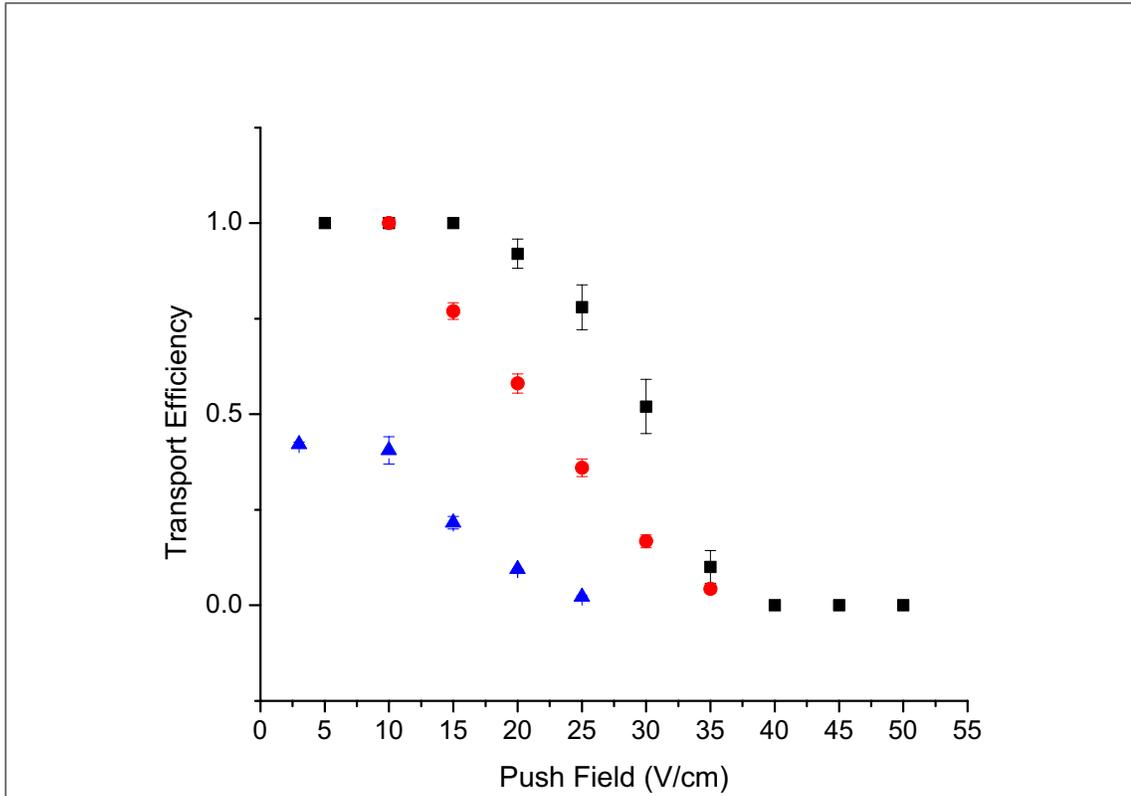
Figure 3.45. Transport efficiency at 60 torr for a varying push field for experiment (blue triangles), space charge simulations (red circles), and HS-collision simulations (black squares). Rf carpet parameters: Rf voltage at discharge limit at 2 MHz, Drag Field = 3 V/cm, Push Field = 3 V/cm, Experimental transport distance = 8 cm, Simulated transport distance = 5 cm,  $I(Carp) = 2$  nA.
