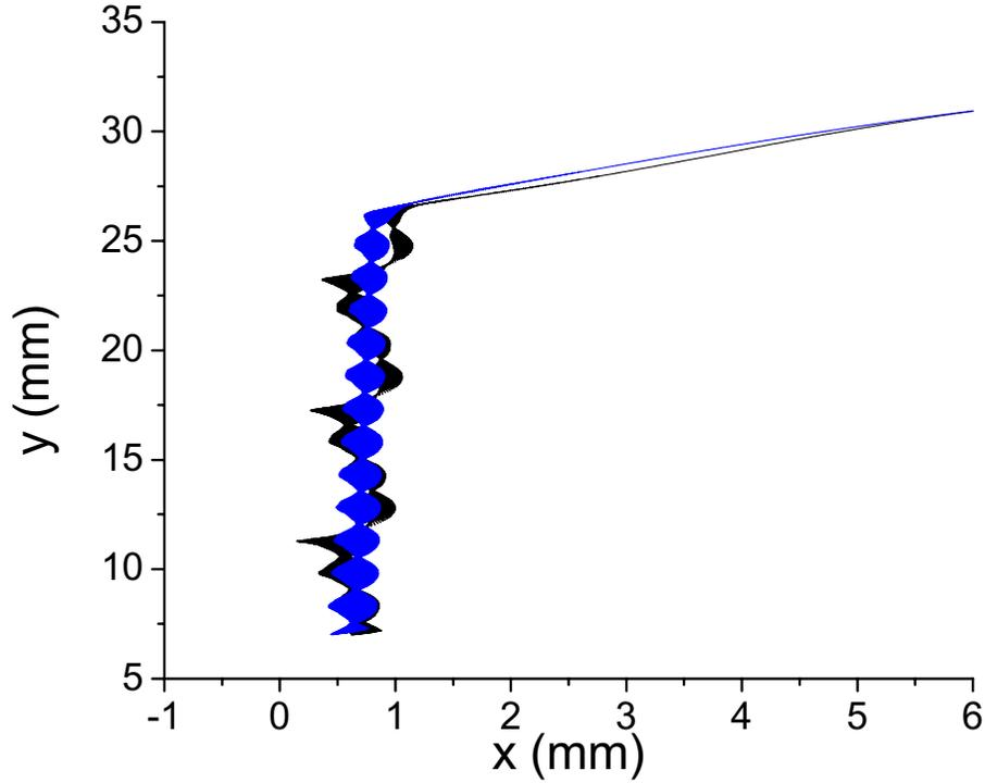
Figure 2.11. Trajectories from a rf carpet simulation with  $a=1.5$ ,  $\gamma=0.7$  with simulation parameters shown in Table 2.3. The carpet electrodes (not shown) are located at  $x=0$  and the push electrodes (not shown) are located at  $x=20$ . Blue line: No electrode grouping. Black line: Electrode grouping of 4.
