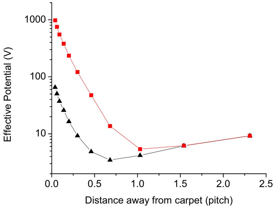
Figure 2.7. Calculated effective potential for a rf carpet ( $a = 0.5$  mm and  $\gamma = 0.5$ ) as a function of distance away from the carpet superimposed with the static potentials from an electric field perpendicular to the carpet electrodes ( $2$  V/mm). For an ion with  $A = 85$  amu ion at  $2$  MHz and a rf voltage of  $200$  V<sub>RF,pk-pk</sub> Black Curve: 100 mbar. Red Curve: 10 mbar.
