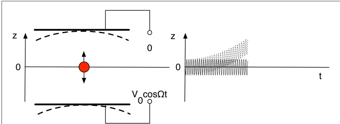
Figure 2.1. Illustration of effective force on an ion in an inhomogeneous electric rf-field. Left: Ion placed in between a set of parallel plates (solid) and curved plates (dotted). Right: Ion's position over time for the parallel plate (solid) case and curved plate (dotted) case.
