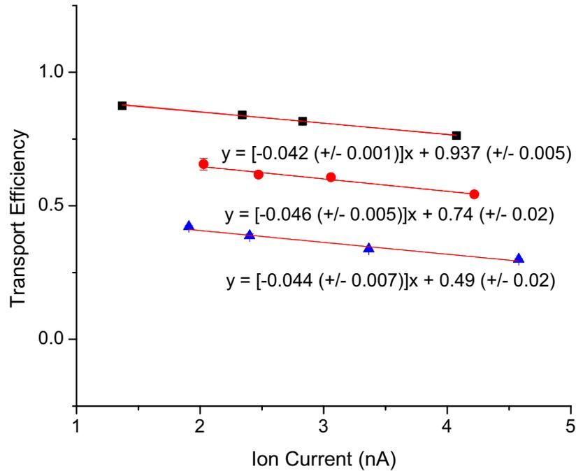
Figure 3.42. Measured transport efficiency at 30 torr with varying  $I(Carp)$  for a push field of 10 V/cm (black squares), 15 V/cm (red circles), and 20 V/cm (blue triangles). Rf carpet parameters: Rf voltage at discharge limit at 2 MHz, Drag Field = 3 V/cm, Transport Distance = 8 cm.
