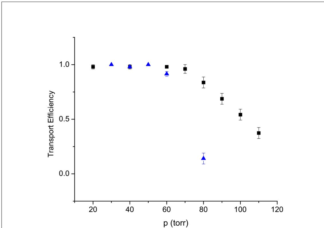
Figure 3.34. Comparison of transport efficiency over the operating pressure regime of the cyclotron gas stopper for a rf driving frequency of 2 MHz (blue triangles) and 3.47 MHz (black squares). Rf carpet parameters: Rf voltage at discharge limit, Drag Field = 3 V/cm, Push Field = 3 V/cm, Transport Distance = 16 cm, Pitch = 0.38 mm,  $\gamma = 0.5$ ,  $I(Carp) = 700$  pA.
