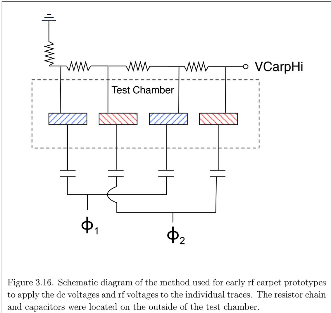
Figure 3.16. Schematic diagram of the method used for early rf carpet prototypes to apply the dc voltages and rf voltages to the individual traces. The resistor chain and capacitors were located on the outside of the test chamber.
