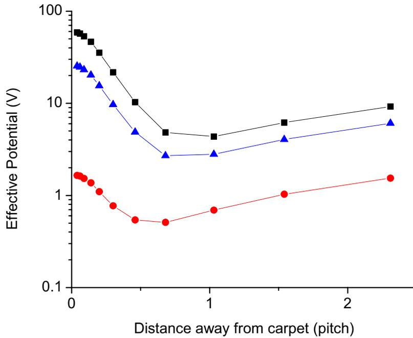
Figure 3.37. Comparison of the calculated effective potential a  $A=85$  ion experiences from a rf carpet with a pitch of 1.5 mm (red circles), 0.38 mm (blue triangles), and 0.25 mm (black squares) in 80 torr of He gas with a driving frequency of 2 MHz, Rf voltage at discharge limit and a push field of 10 V/cm.
