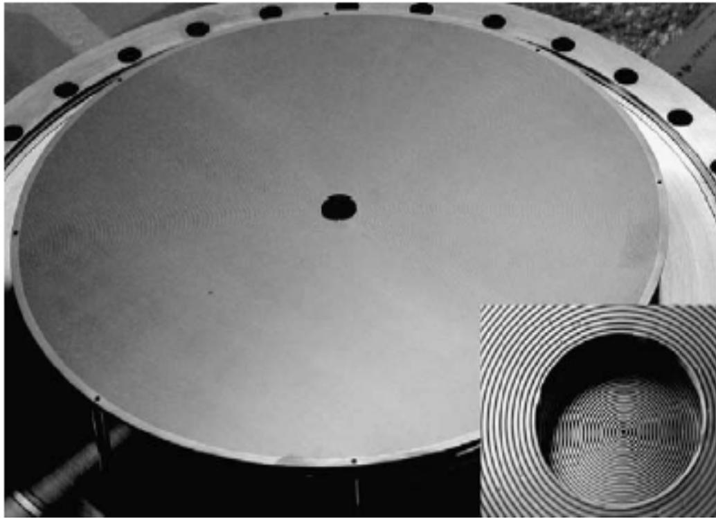
Figure 1.4. Photograph of a ion collection system with a rf carpet from RIKEN [5]. The top electrode system has a diameter of 29 cm with 280 electrodes and a central hole of 10 mm. It is only biased with dc voltages [11] and is used to guide the ions towards the rf carpet (insert). The rf carpet is located below the top electrode system and has a diameter of 3 cm with 43 electrodes and an exit hole of 0.6 mm.
