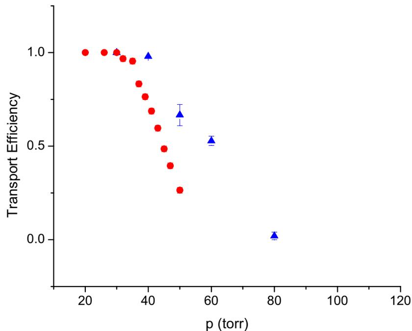
Figure 3.36. Comparison of the transport efficiency for a pitch of 1.5 mm,  $\gamma = 0.7$  (red circles) and a pitch of 0.38 mm,  $\gamma = 0.5$  (blue triangles). Rf carpet parameters: Rf voltage at discharge limit, Drag Field = 3 V/cm, Push Field = 3 V/cm, Transport Distance = 16 cm,  $I(Carp) \geq 2.5$  nA.
