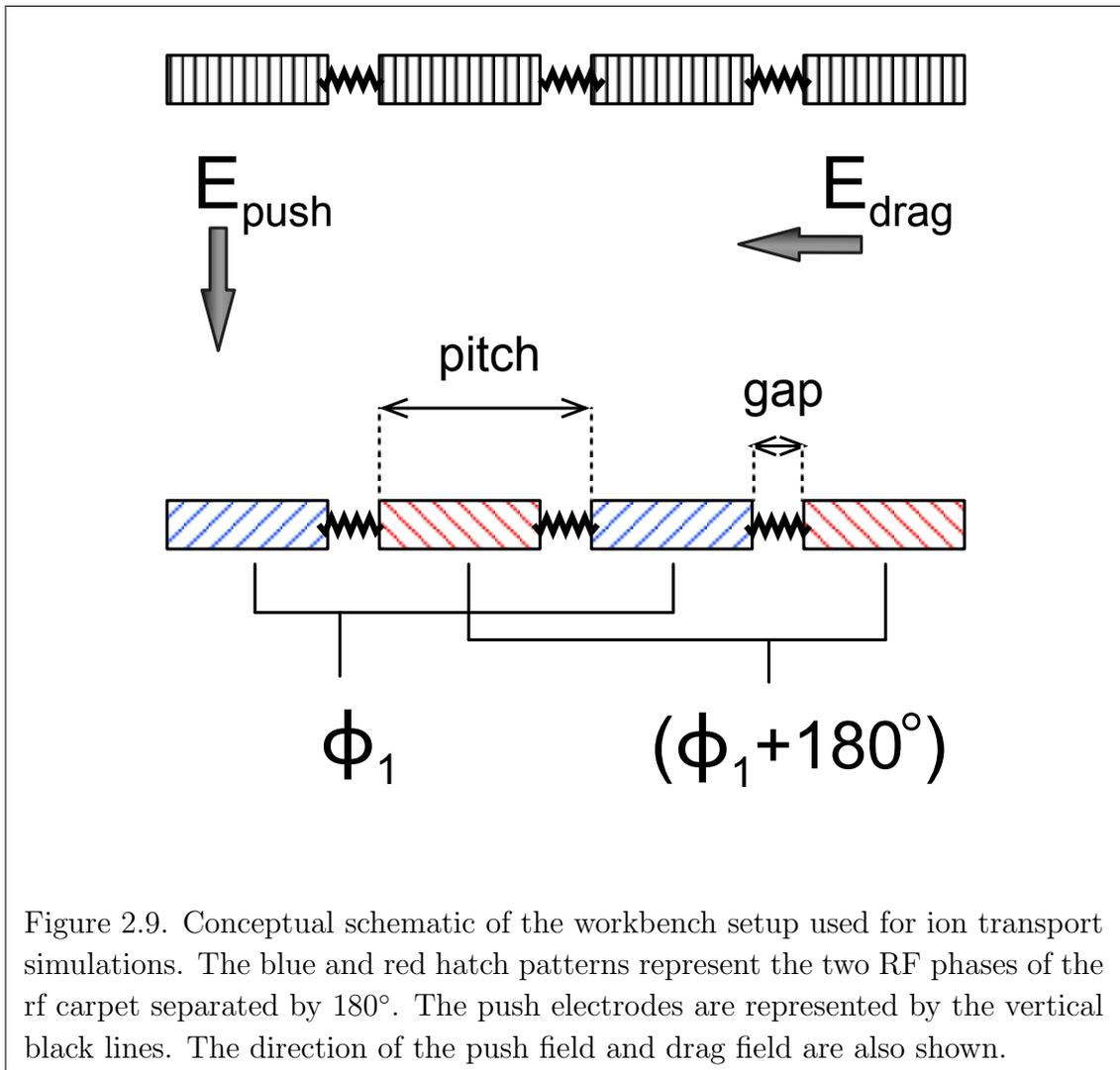
Figure 2.9. Conceptual schematic of the workbench setup used for ion transport simulations. The blue and red hatch patterns represent the two RF phases of the rf carpet separated by  $180^\circ$ . The push electrodes are represented by the vertical black lines. The direction of the push field and drag field are also shown.
