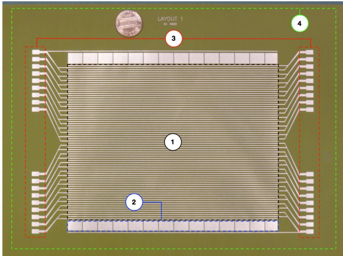
Figure 3.10. A linear carpet design with straight (linear) stripes for the transport area. The different design elements are designated by the numbered areas that are outlined outlined by the colored dashed lines. (1) Dashed black line: transport area; (2) Dashed blue line: segmented ion collection area; (3) Dashed red line: Rf & dc contacts; (4) Dashed green line: clamping area - Kapton (substrate) border. The coin, included for scale, is a US penny.
