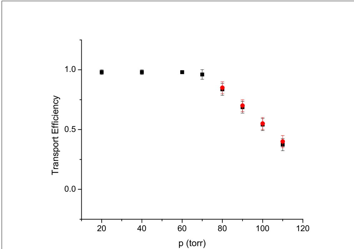
Figure 3.32. Measured (black squares) and predicted (red circles) transport efficiency of the rf carpet over the operating pressure regime of the cyclotron gas stopper. Rf carpet parameters: Rf = 3.47 MHz at discharge limit, Drag Field=3 V/cm, Push Field=3 V/cm, Transport Distance=16 cm, Pitch = 0.38 mm,  $\gamma=0.5$ ,  $I(Carp) = 700$  pA. Black squares: Measured, Red Circles: Predictions.
