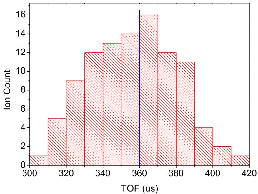
Figure 2.12. Histogram showing the TOF distribution of 100 ions with a collision cross-section of  $2.75\text{E-}19 \times 10^{-19} \text{ m}^2$ . The blue vertical line refers to the TOF according to the ion mobility.
