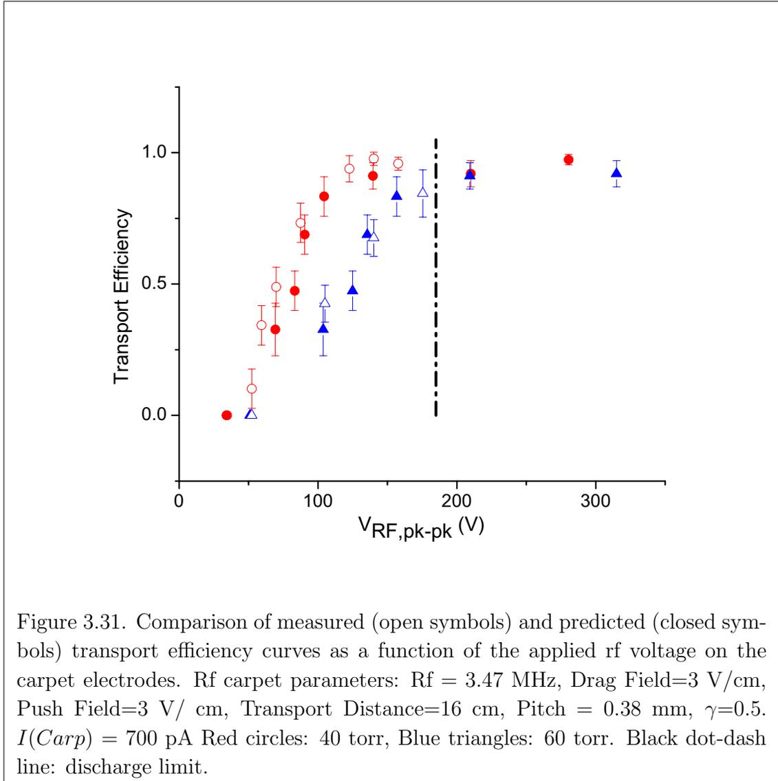
efficiencies and the predicted transport efficiencies were in good agreement with each other and provided a useful tool to verify if transport efficiency measurements were consistent amongst each other at different pressures for identical rf carpet parameters over time.
