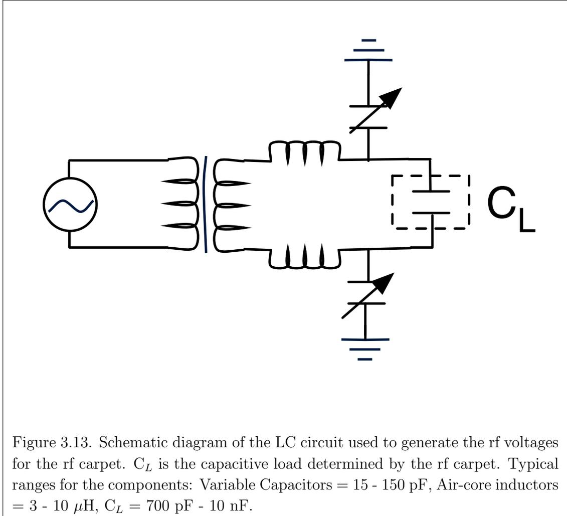
Figure 3.13. Schematic diagram of the LC circuit used to generate the rf voltages for the rf carpet.  $C_L$  is the capacitive load determined by the rf carpet. Typical ranges for the components: Variable Capacitors = 15 - 150 pF, Air-core inductors = 3 - 10  $\mu\text{H}$ ,  $C_L = 700 \text{ pF} - 10 \text{ nF}$ .
