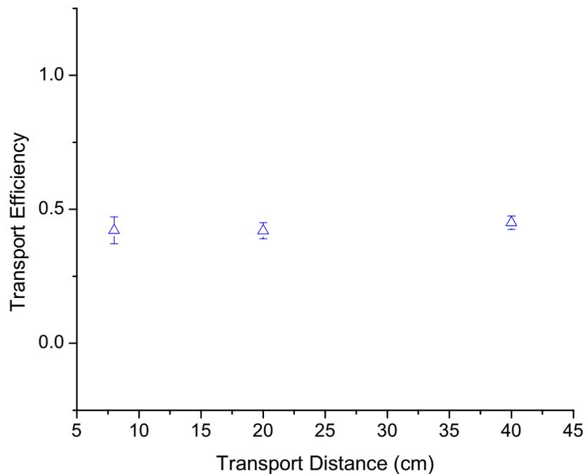
Figure 3.41. Measured transport efficiency at 60 torr with  $I(Carp) = 2.0$  nA over different transport distances across the rf carpet. Rf carpet parameters: Rf voltage at discharge limit at 2 MHz, Drag Field = 3 V/cm, Push Field = 3 V/cm.
