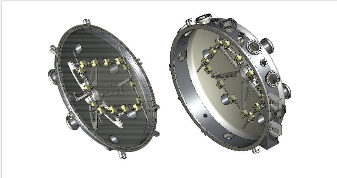
Figure 3.3. Mechanical drawing of the clamping method that allowed for easier modification of the carpet electrodes without having to redo the clamping process. The carpet electrodes are represented by the opaque grey rectangular sheets. Left: Frame on the door side. Right: Frame on the chamber side.
