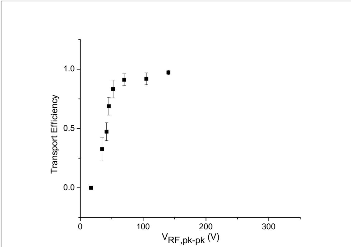
Figure 3.29. Measured transport efficiency as a response to the applied rf voltage on the carpet electrodes. Experimental parameters: Chamber pressure=20 torr, Rf = 3.47 MHz, Drag Field=3 V/cm, Push Field=3 V/cm, Transport Distance=16 cm, Pitch = 0.38 mm,  $\gamma=0.5$ ,  $I(Carp) = 700$  pA.
