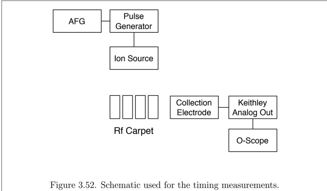
obtained. A schematic of the experimental setup is shown in Fig. 3.52.
