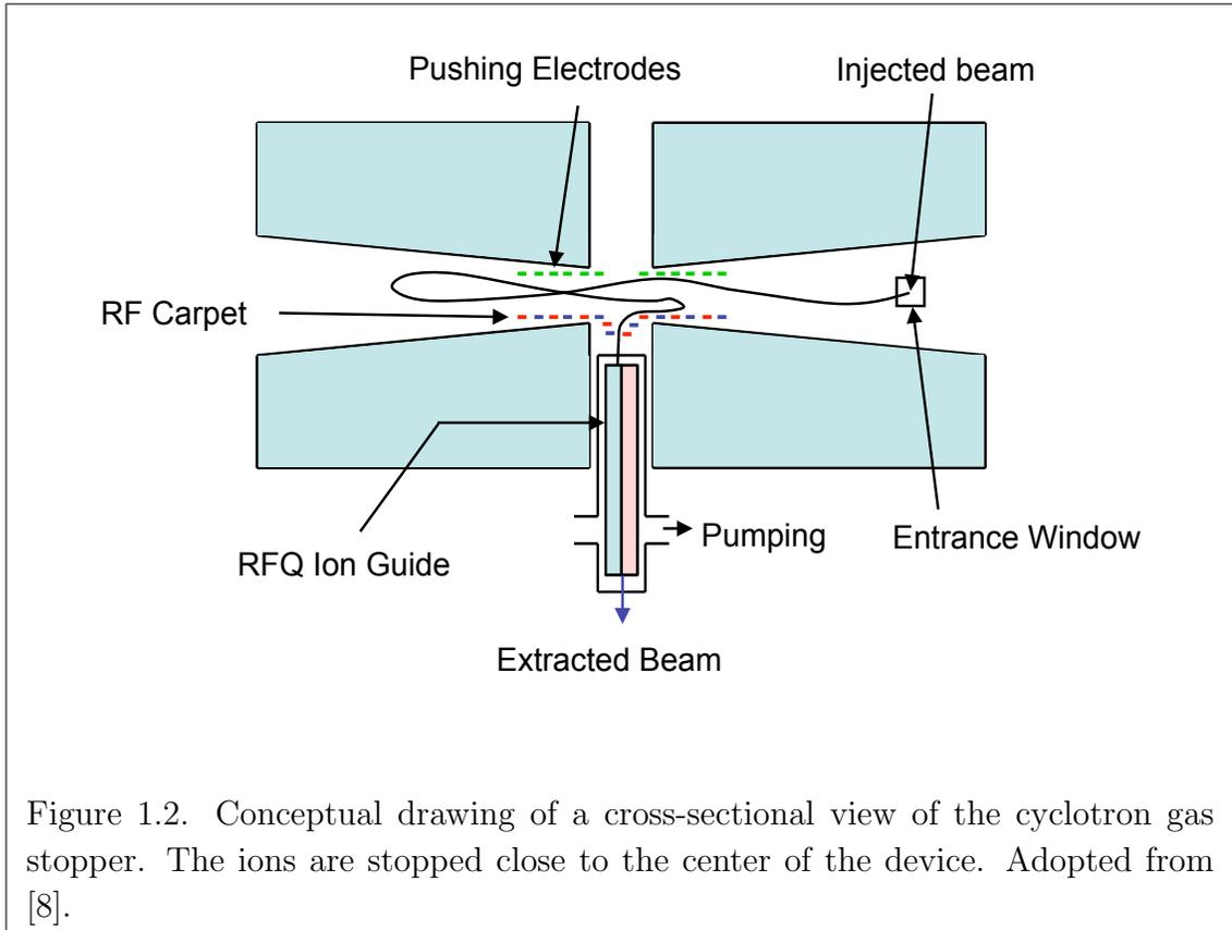
such a device is shown in Fig. 1.2. The energetic beam is injected into the system and encounters an adjustable solid degrader to degrade the beam, so that the resultant beam follows an inwards spiral path and is thermalized near the center of the magnet. A sample trajectory of an ion in the system along with the distribution of stopped ions near the center of the system from simulations is shown in Fig. 1.3.
