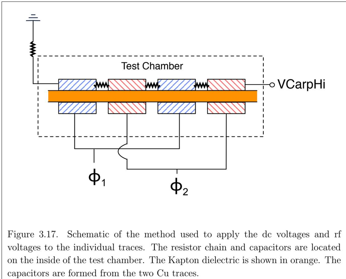
capacitively coupled to the topside (transport side) of the flex circuit. The dc voltages were generated with surface mount resistors as in section 3.4.2 and applied directly to the topside of the carpet. This is equivalent to the schematic in Fig. 3.16, but avoids the installation of individual capacitors.
