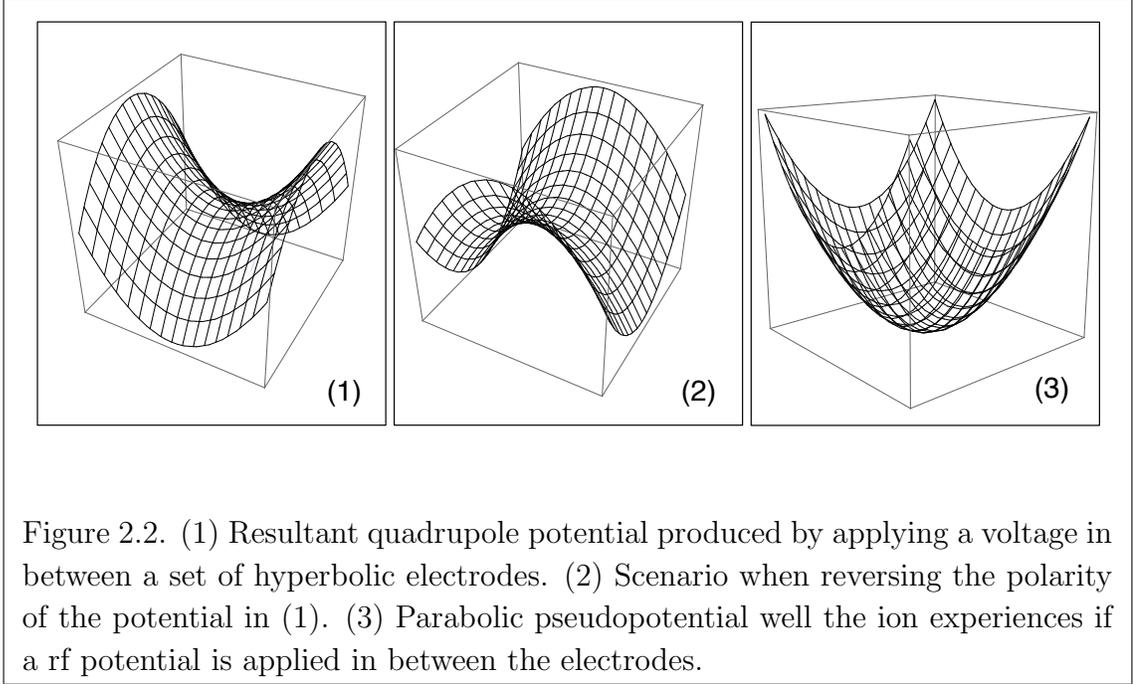
$$V_{eff} = \frac{e}{m} \frac{V^2 (x^2 + y^2)}{\Omega r_0^4} \quad (2.9)$$
