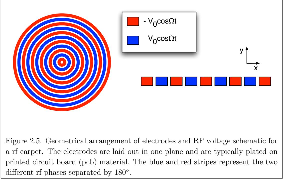
future discussions, the gap,  $g$  is defined as the spacing between adjacent electrodes and the pitch,  $a$ , is defined as the sum of the electrode width and the gap. From [17],
