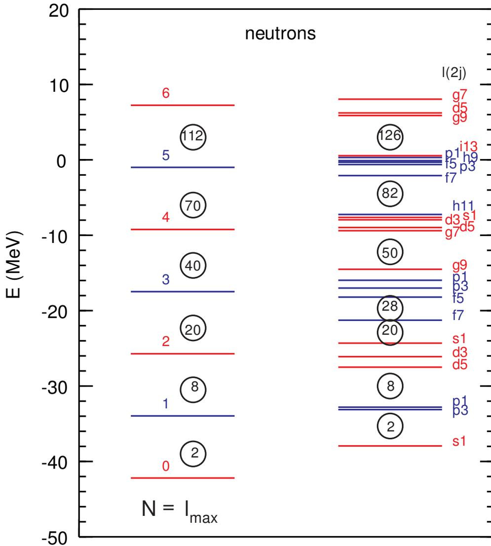
Figure 1.2: Schematic view of the single particle states in  $^{132}\text{Sn}$  with a harmonic oscillator mean field and the splitting that occurs with the addition of a strong spin-orbit potential. For interpretation of the references to color in this and all other figures, the reader is referred to the electronic version of this dissertation.
