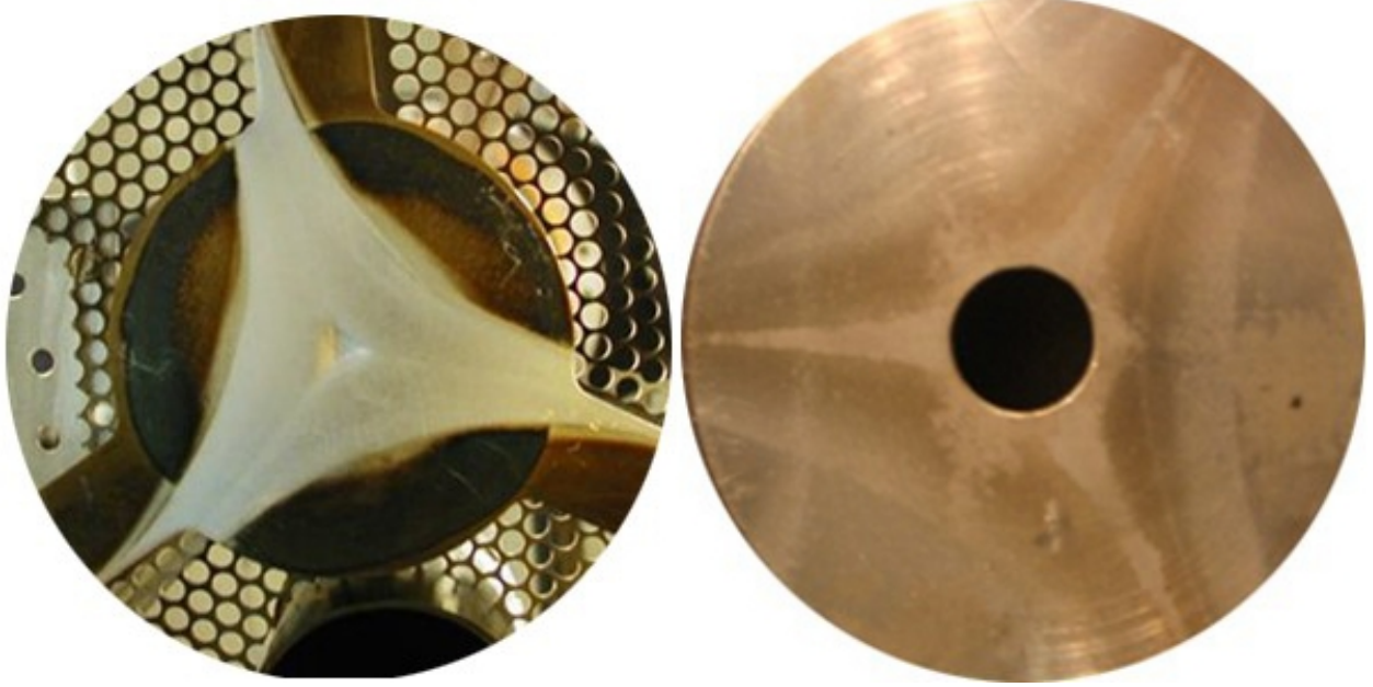
Figure 6.2: Plasma sputter marks inside VENUS. Left: The biased disk exhibits a large star structure and a smaller clear triangle of about 5 mm height etched into the plate. Right: The same (now rotated) discolorations are seen, however the triangle would be inside the extraction aperture.
