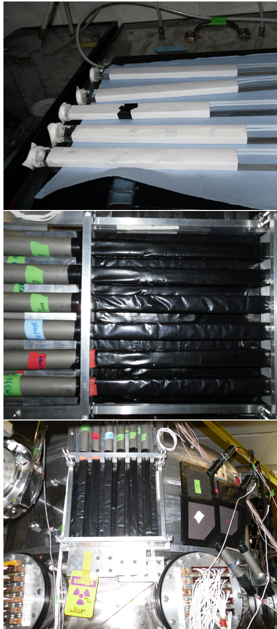
Figure 2.22: (From top to bottom) The Veto bars after they have been polished and partially wrapped. The complete array of the Proton Veto bars in their mount. All Proton Veto bars and paddles in experimental setup.
