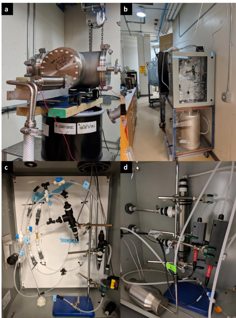
Figure 2.14: Images of the Isotope Harvesting System for the High Intensity Proton Irradiation Pictures showing the target at the end of the cyclotron line (a), the water system in secondary containment sitting behind a shielding wall (b), the inside of the aqueous chemistry box (c), and the inside of the hydrogen peroxide decomposition box (d).
