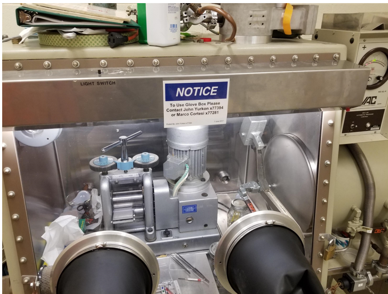
Figure 3.21: Interior of glove box used for lithium target preparation. Mason jars used for the transfer of materials are visible, as well as the metal roller used to achieve the desired thickness of the self-supporting lithium.
