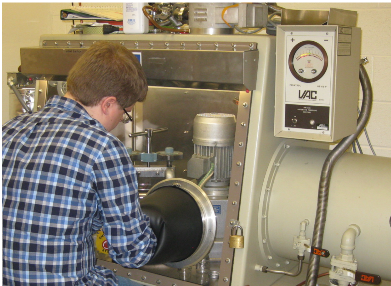
Figure 3.20: Preparation of the lithium target in a glove box filled with Argon.
