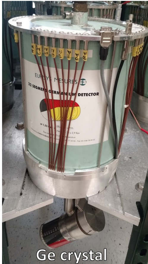
Figure 3.6: A germanium detector from SeGA. The large green cylinder is the liquid nitrogen reservoir, the preamplifiers are directly below the dewar inside the casing, and the germanium crystal itself is the inside the cylinder at the bottom of the image. The figure is from Ref. [74].
