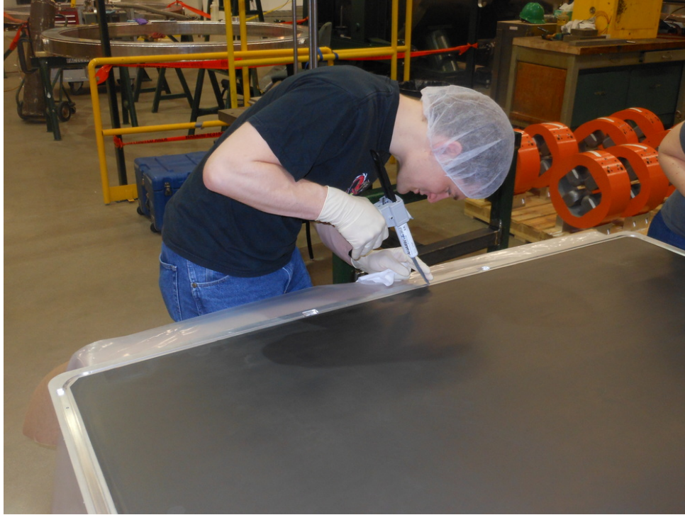
Figure 2.35: Justin Estee (GS) applies epoxy to the cathode plate.
