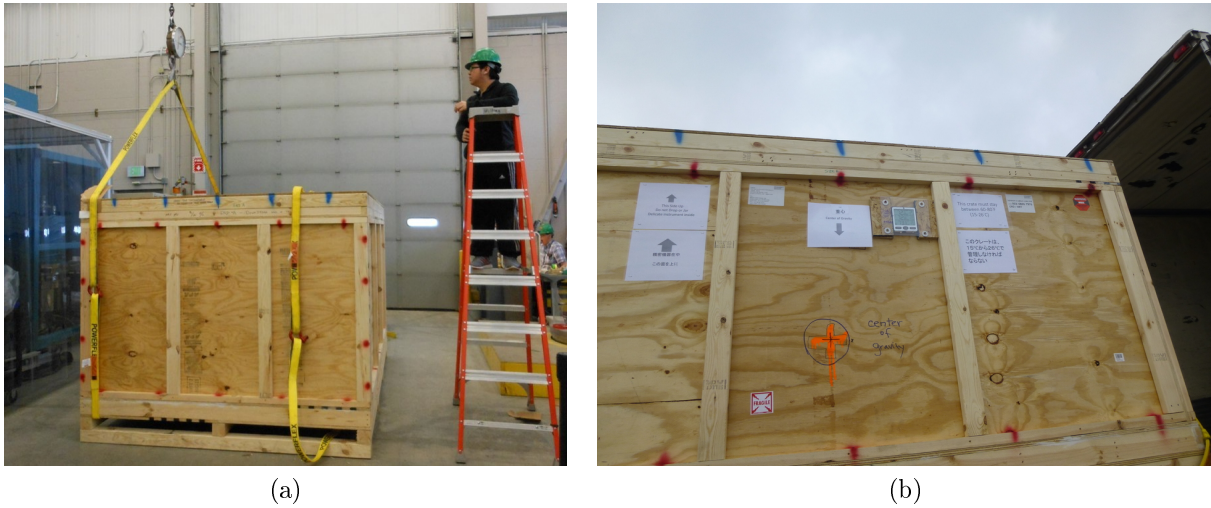
Figure 2.47: Weighing the packed crate. In addition to the overall weight, the crate was measured from each end (a) allowing us to determine and mark the center of gravity (marked with orange paint in (b)).
