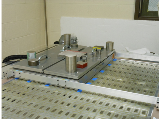
Figure 2.14: Vacuum table in use for pad plane installation.
