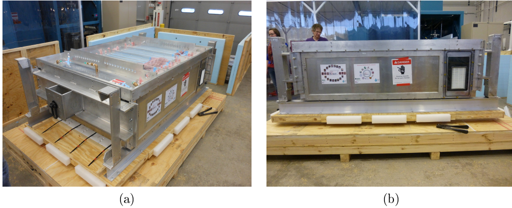
Figure 2.45: The TPC installed on the crate platform. The bed of phase change material is visible in (a), and the side profile shown in (b) shows one of the HEPA window filters.
