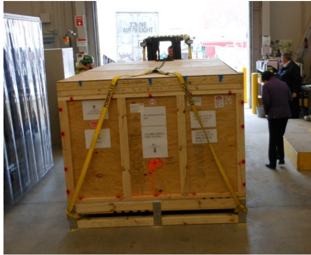
Figure 2.48: Strapping the crate to the forklift at the NSCL. Two lifting straps (yellow) are secured to the forklift with a chain, visible on the top of the crate.
