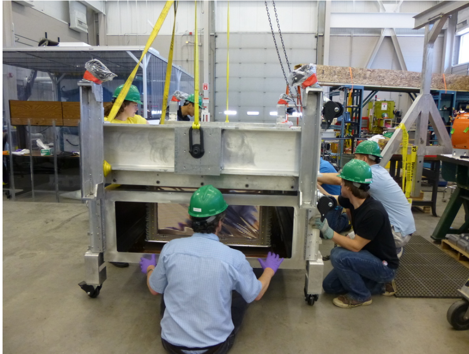
Figure 2.50: Lifting the top plate and field cage out of the enclosure.
