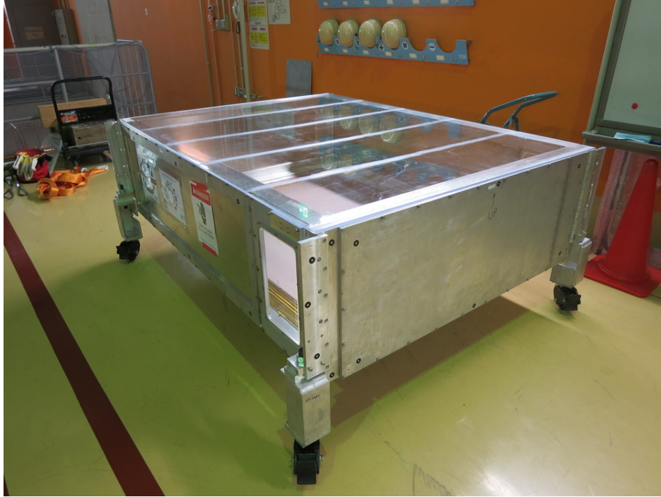
Figure 2.42: TPC enclosure with top plate removed.
