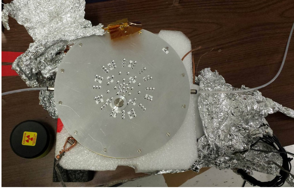
Figure 3.4: The MICROMEAS being operated in “pancake” mode. By shortening the active volume of the gas, we were able to use an ^{55}\text{Fe} X-ray source to characterize the performance of individual detector pads.
