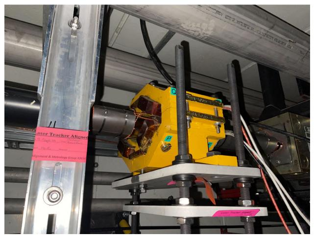
Figure 7.2 Newly installed compensation sextupoles in the 620 section.
