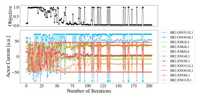
Figure 5.8 Summary for Bayesian optimization of resonance compensation applied to Ring 2 in the CERN PSB.
