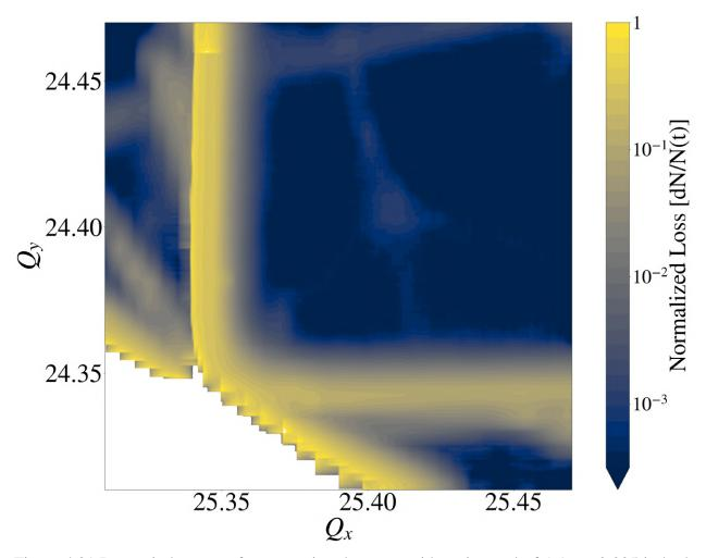
Figure 4.21 Dynamic loss map from ramping the tunes with an interval of  $\Delta Q_u = 0.005$  in both directions. The directions of the scan are from left to right and top to bottom. The results are superimposed in this plot.
