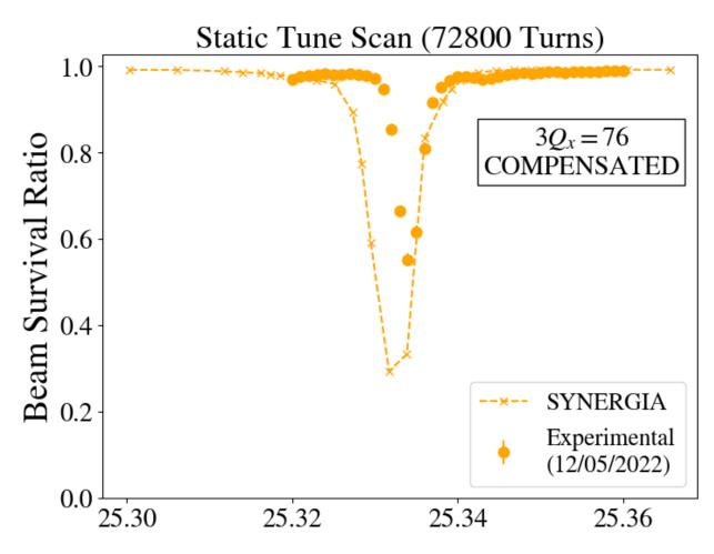
Figure 4.25 Plot for static tune scan for the machine with  $3Q_x$  compensation, including a comparison between experimental data and SYNERGIA simulations.
