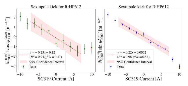
Figure 4.15 Real and imaginary part of  $h_{3000}$  as a function of current fed to compensation sextupole SC319. Measurement is shown for R:HP612 data.
