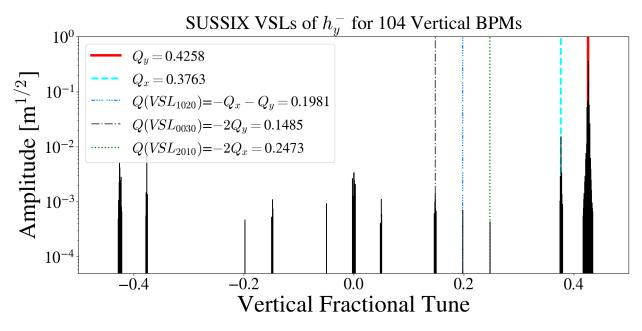
Figure 4.7 Spectral lines of  $h_y^-$  calculated with SUSSIX [42]. The  $h_y^-$  signal was reconstructed for the 104 Vertical BPMs. The spectrum for all BPMs is superimposed in this plot.
