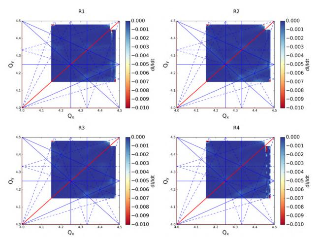
Figure 5.13 Dynamic loss maps for the four rings in the PS Booster with the best configuration from the Bayesian optimization of the resonance compensation. The plots are an average of scanning in 4 directions. Plot provided by F. Asvesta.
