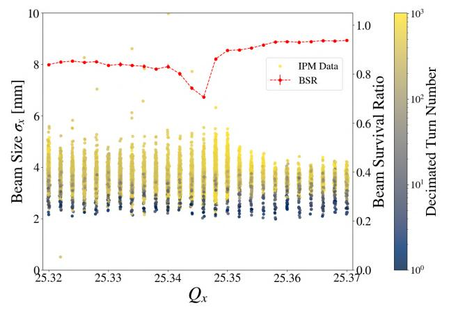
Figure 6.6 Static tune scan at an equivalent intensity of 8 Booster turns or approximately 3e10 ppb.
