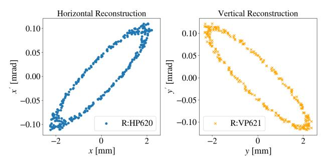
Figure 4.4 Phase space coordinates reconstruction for two neighboring BPMs—one horizontal R:HP620 and one vertical R:VP621—windowed for 300 turns.
