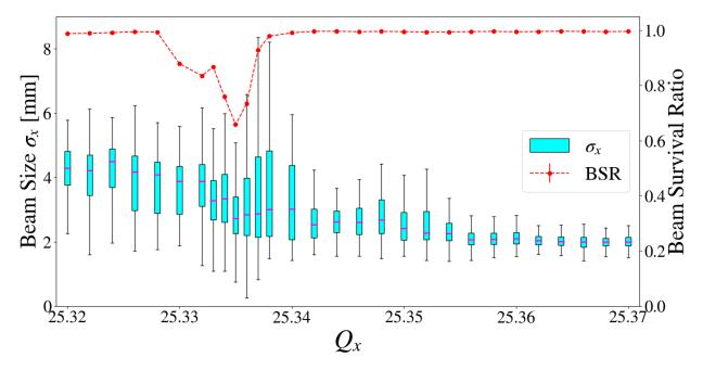
Figure 6.12 Static tune scan with beam survival ratio and IPM data box plots with  $3Q_x$  compensation, transverse dampers ON and 2 Booster Turns of equivalent intensity or approximately 0.5e10 ppb.
