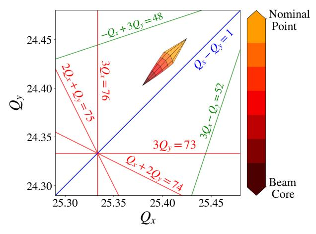
Figure 2.5 Tune footprint for a Gaussian beam in the Recycler Ring at an intensity of 5e10 particles per bunch created with PySCRDT.
