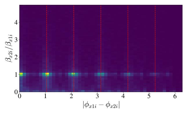
Figure 4.29 2D Histogram of optimum lattice locations where the compensating  $K_2$  coefficients with the two new sextupoles are minimized. Red dashed lines correspond to thirds of  $\pi$ .
