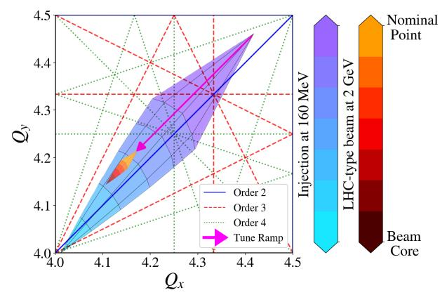
Figure 5.2 Operational tune footprint for PSB beam at injection (cool color map) and footprint after the beam has been accelerated to 2 GeV (warm color map). During acceleration, there is a tune ramp illustrated with the fuchsia arrow.
