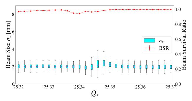
Figure 6.13 Static tune scan with beam survival ratio and IPM data box plots with  $3Q_x$  compensation, transverse dampers OFF and 2 Booster Turns of equivalent intensity or approximately 0.5e10 ppb.
