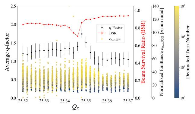
Figure 6.10 Static tune scan with beam survival ratio (BSR), average q-factor for the q-Gaussian fits, and normalized emittance at an equivalent intensity of 8 Booster turns or approximately 3e10 ppb.
