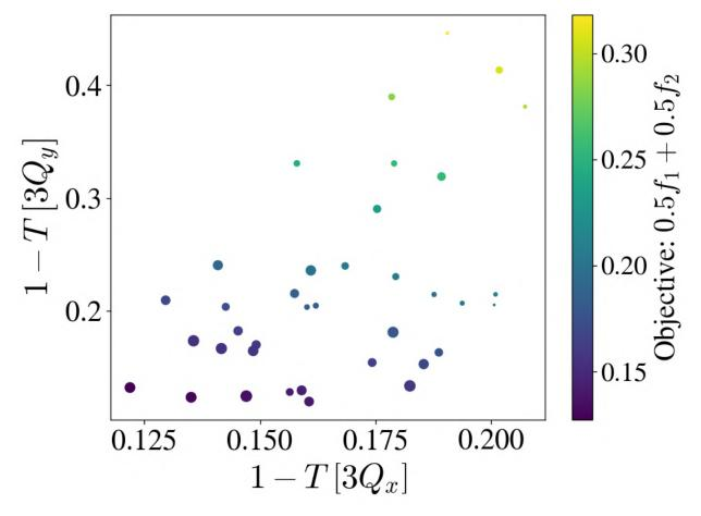
Figure 4.19 Multiobjective Nelder-Mead optimization of the transmission through  $3Q_x$  and  $3Q_y$ . The objective function to be minimized was defined as an equally weighted sum of both minus transmissions—corresponding to the fractional losses through the resonance lines.
