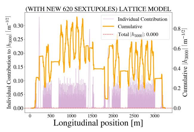
Figure 4.32 Distribution of the  $h_{3000}$  term around the ring with individual contributions from each relevant element and the cumulative sum from an arbitrary starting point. This calculation includes the new 620 sextupoles powered at the correct currents to simultaneously cancel out  $h_{3000}$  and  $h_{1020}$ .
