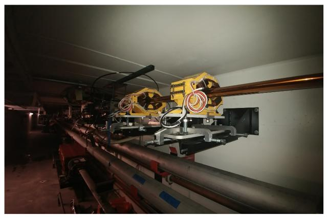
Figure 3.12 Picture of compensation sextupoles (yellow magnets on top) installed in the Recycler Ring. Picture provided by Dr. Robert Ainsworth.
