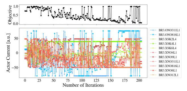
Figure 5.9 Summary for the first instance of Bayesian optimization towards resonance compensation applied to Ring 3 in the CERN PSB.
