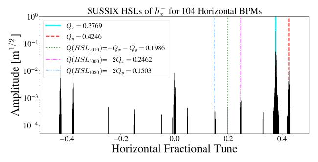
Figure 4.6 Spectral lines of  $h_x^-$  calculated with SUSSIX [42]. The  $h_x^-$  signal was reconstructed for the 104 Horizontal BPMs. The spectrum for all BPMs is superimposed in this plot.
