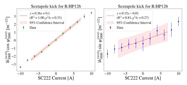
Figure 4.14 Real and imaginary part of  $h_{3000}$  as a function of current fed to compensation sextupole SC222. Measurement is shown for R:HP126 data.
