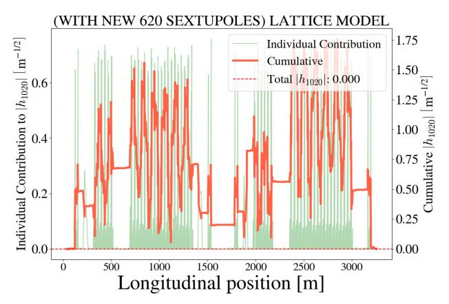
Figure 4.33 Distribution of the  $h_{1020}$  term around the ring with individual contributions from each relevant element and the cumulative sum from an arbitrary starting point. This calculation includes the new 620 sextupoles powered at the correct currents to simultaneously cancel out  $h_{3000}$  and  $h_{1020}$ .
