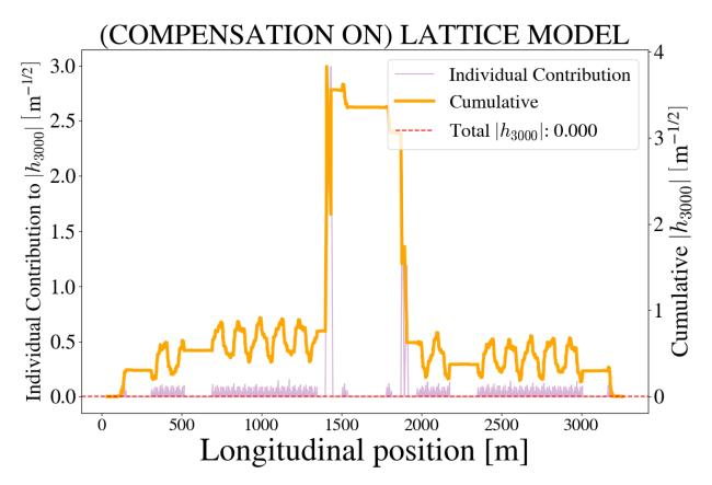
Figure 4.12 Distribution of the  $h_{3000}$  term around the ring with individual contributions from each relevant element and the cumulative sum from an arbitrary starting point. This sum is done with existing sextupoles powered at the correct currents to simultaneously cancel out  $h_{3000}$  and  $h_{1020}$ .
