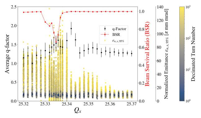
Figure 6.14 Static tune scan with beam survival ratio (BSR), average q-factor for the q-Gaussian fits, and normalized emittance with  $3Q_x$  compensation ON, transverse dampers ON and 2 Booster Turns of equivalent intensity or approximately 0.5e10 ppb.
