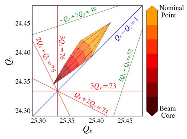
Figure 3.8 Approximate operational tune footprint at high intensities, i.e., 1e11 particles per bunch.
