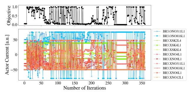
Figure 5.10 Summary for the second instance of Bayesian optimization of resonance compensation applied to Ring 3 in the CERN PSB. This second optimization instance was trained with the data from the first instance.
