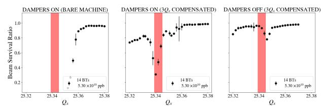
Figure 7.1 Transverse damper effect on resonance compensation for bare machine + dampers ON,  $3Q_x$  compensated + dampers ON, and  $3Q_x$  compensated + dampers OFF configuration. The red band corresponds to the  $3Q_x$  stop band at an intensity of 0.5 ppb with dampers ON.
