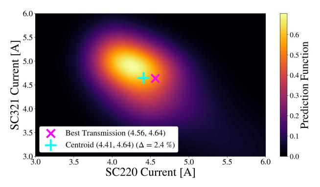
Figure 4.17 Prediction function built from the best R-squared statistics BPMs to predict the best global currents for  $h_{3000}$  compensation.
