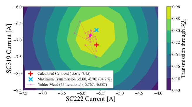
Figure 4.18 Nelder-Mead optimization from an instance where the response matrix prediction was used as the initial point. The contour plot shows the transmission through  $3Q_x$  as a function of the currents.
