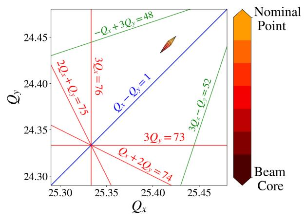
Figure 2.4 Approximate operational tune footprint at low intensities calculated with PySCRDT [22], i.e., 1e10 particles per bunch.
