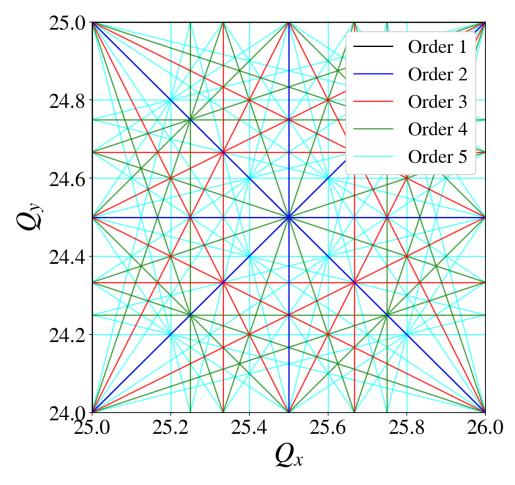
Figure 2.3 Tune diagram with resonance lines up to fifth order, enclosing the operation point of the Recycler Ring.
