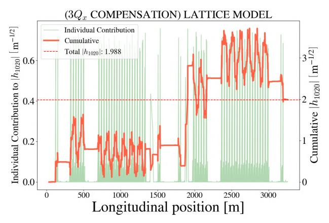
Figure 4.11 Distribution of the  $h_{1020}$  term around the ring with individual contributions from each relevant element and the cumulative sum from an arbitrary starting point when correction elements are set to compensate  $3Q_x = 76$ , i.e.,  $h_{3000} = 0$ .
