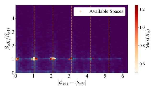
Figure 4.30 2D Histogram of optimum lattice locations where the compensating  $K_2$  coefficients with the two new sextupoles are minimized with available drift spaces candidates scattered on top of it.
