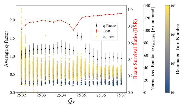
Figure 6.11 Static tune scan with beam survival ratio (BSR), average q-factor for the q-Gaussian fits, and normalized emittance at an equivalent intensity of 14 Booster turns or approximately 4.5e10 ppb.
