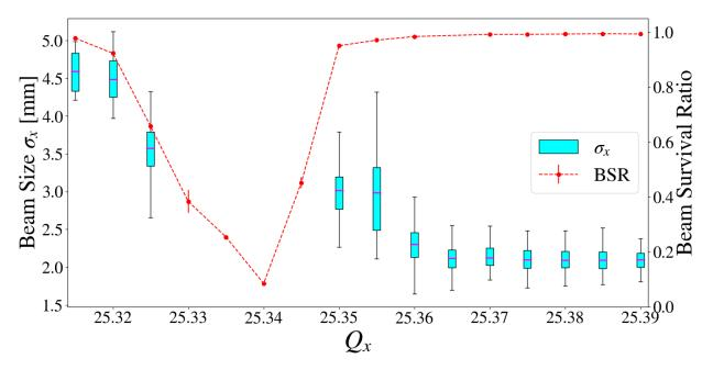
Figure 4.26 Static tune scan with beam survival ratio and IPM data box plots for the bare machine at 2 Booster Turns of equivalent intensity.
