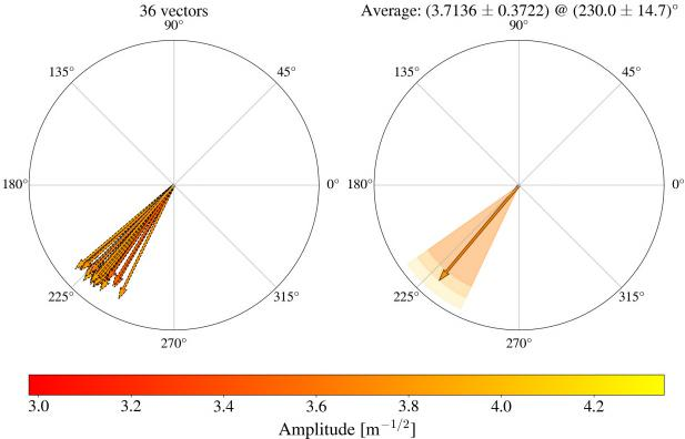
Figure 4.8 Polar plot for the measurement of  $h_{3000}$  for 36 measurements at horizontal BPM R:HP620. For every BPM, measurements like those presented in Fig. 4.8 are done. In the case of the
