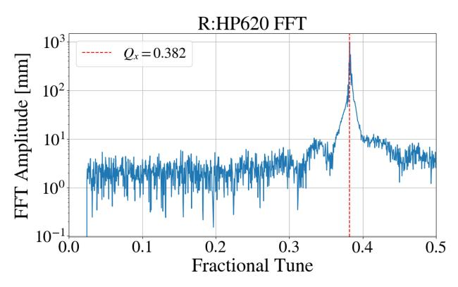
Figure 3.10 Fast Fourier Transform amplitude for the turn-by-turn data presented in Fig. 3.9.
