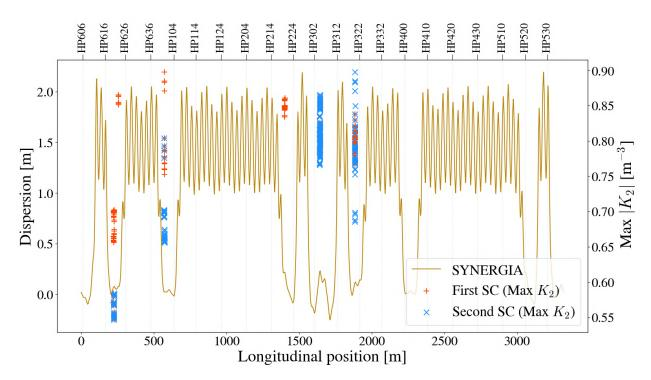
Figure 4.31 Dispersion function of the Recycler Ring with possible new locations to introduce a pair of sextupole magnets that cancel out  $h_{3000}$  and  $h_{1020}$  simultaneously. The right y-axis shows the maximum compensation  $K_2$  coefficient needed with these new candidates.
