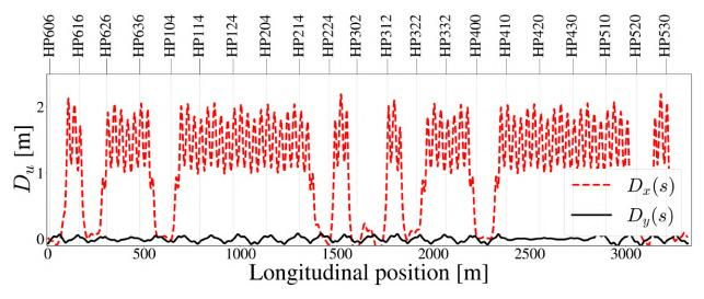
Figure 3.6 Dispersion functions for the Recycler Ring lattice tuned to  $Q_x = 25.44$  and  $Q_y = 24.39$ . Lattice functions are calculated from the lattice file using SYNERGIA.
