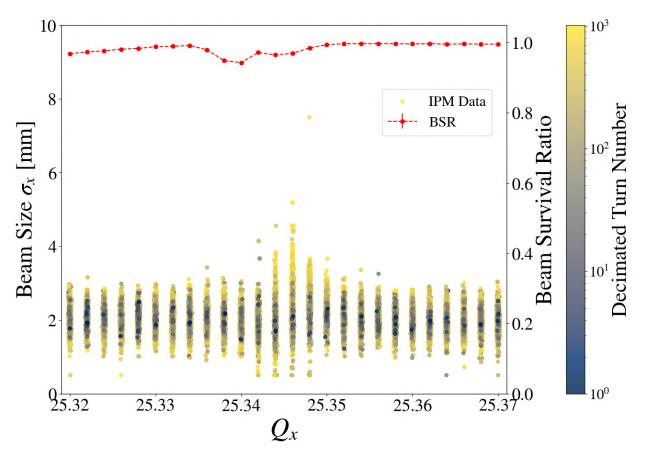
Figure 6.5 Static tune scan at an equivalent intensity of 2 Booster turns or approximately 0.5e10 ppb.
