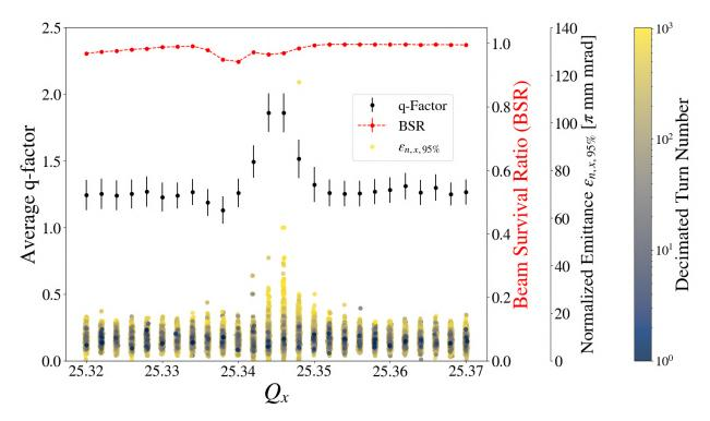
Figure 6.9 Static tune scan with beam survival ratio (BSR), average q-factor for the q-Gaussian fits, and normalized emittance at an equivalent intensity of 2 Booster turns or approximately 0.5e10 ppb.
