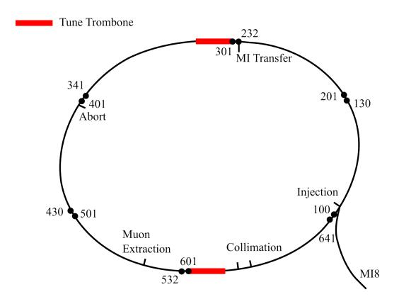
Figure 3.4 Schematic layout of the Recycler Ring and its corresponding sections. Original plot provided by R. Ainsworth, first published on Ref. [32].
