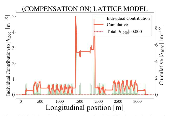
Figure 4.13 Distribution of the  $h_{1020}$  term around the ring with individual contributions from each relevant element and the cumulative sum from an arbitrary starting point. This distribution is with existing sextupoles powered at the correct currents to simultaneously cancel out  $h_{3000}$  and  $h_{1020}$ .
