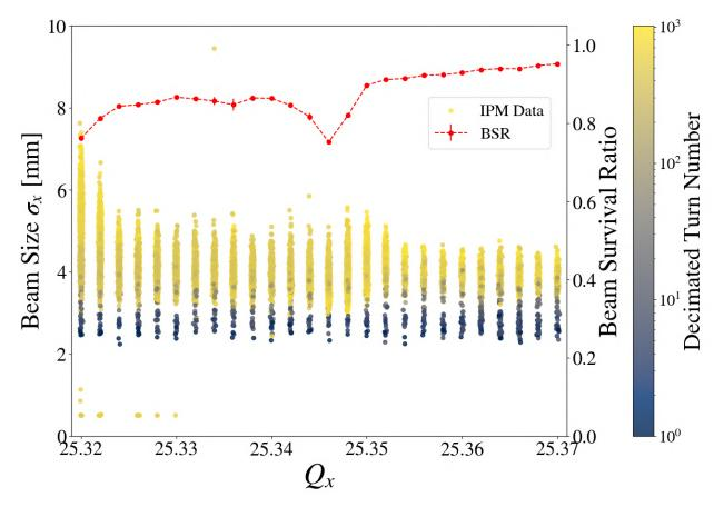
Figure 6.7 Static tune scan at an equivalent intensity of 14 Booster turns or approximately 4.5e10 ppb.
