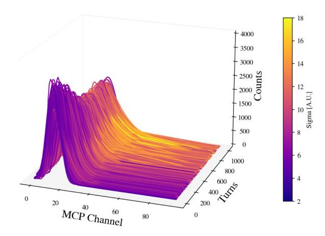
Figure 3.11 Reconstructed beam profile for the horizontal plane assuming Gaussian distributions along 1024 turns for an arbitrary beam in the Recycler Ring.
