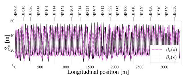
Figure 3.5 Beta functions for the Recycler Ring lattice tuned to  $Q_x = 25.44$  and  $Q_y = 24.39$ . Lattice functions are calculated from the lattice file using SYNERGIA.
