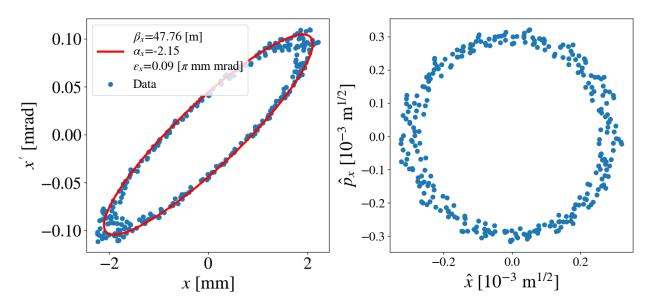
Figure 4.5 Reconstructed phase space data with the best ellipse fit (left plot). The right plot shows the reconstructed normalized phase space using Eq. 2.13 with the Twiss parameters, as estimated from the ellipse fit. This data corresponds to the horizontal data shown in Fig. 4.4 for the R:HP620 BPM.
