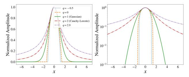
Figure 6.3 Several q-Gaussian distributions for different q parameters normalized to unit amplitude and with a scale parameter of  $\sigma = 1$ . The left plot uses linear scaling, and the right plot uses logarithmic scaling for the y-axis.
