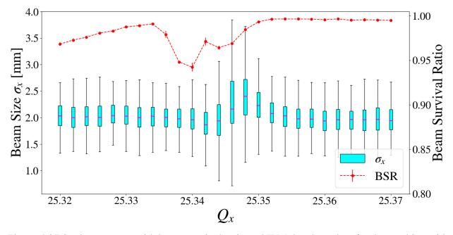
Figure 4.27 Static tune scan with beam survival ratio and IPM data box plots for the machine with  $3Q_x$  compensation at 2 Booster Turns of equivalent intensity.
