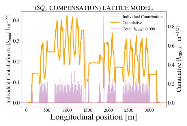
Figure 4.10 Distribution of the  $h_{3000}$  term around the ring with individual contributions from each relevant element and the cumulative sum from an arbitrary starting point when correction elements are set to compensate  $3Q_x = 76$ , i.e.,  $h_{3000} = 0$ .
