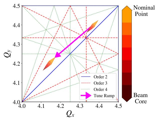
Figure 5.5 Experimental setup of the tune diagram dynamics for optimizing resonance compensation used in the PS Booster.
