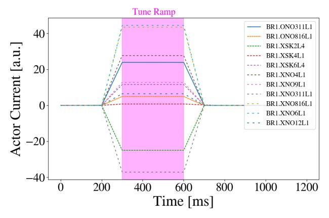
Figure 5.6 Waveform for the currents fed to the correctors (actors) as a function of time in the study cycle for one particular iteration of an arbitrary optimization instance.
