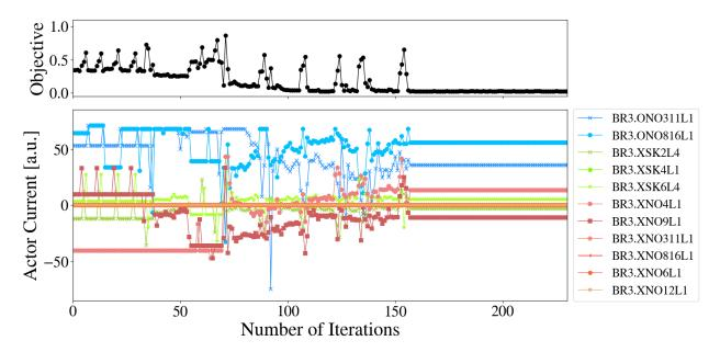
Figure 5.12 Summary for BOBYQA optimization of resonance compensation applied to Ring 3 in the CERN PSB for BCMS (Bunch Compression Merging and Splitting) beam.
