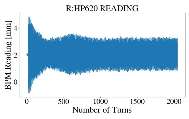
Figure 3.9 BPM turn-by-turn data for an arbitrary kick at horizontal BPM R:HP620.
