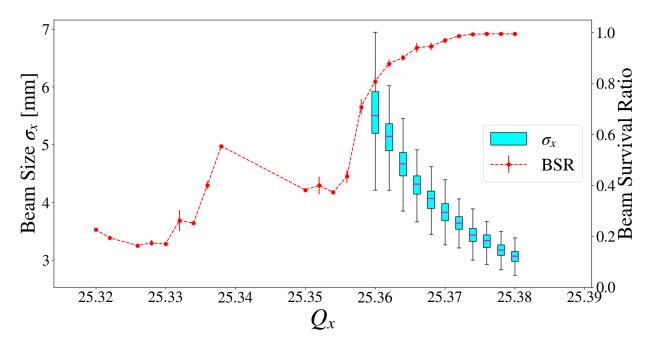
Figure 6.4 Static tune scan at an equivalent intensity of 14 Booster turns or approximately 4.5e10 ppb with no  $3Q_x$  compensation and transverse dampers on.
