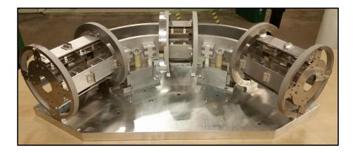
Figure 5.3: 115° cylindrical bender, with integrated electrostatic quadrupole doublets on each end and a quadrupole singlet in the middle for transverse beam focusing.
