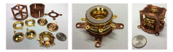
Figure 5.7: SIPT Penning trap electrodes before assembly (left), partway through assembly (middle) and after assembly (right).
