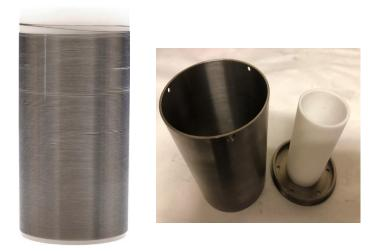
Figure 5.16: 600  $\mu$ H NbTi inductor coil (left) and NbTi inductor case (right) used for the high-Q SIPT FT-ICR detection circuit. The inductor coil consists of 194 turns of 250  $\mu$ m NbTi wire with tubular Teflon coating wrapped around a Teflon core. The windings were then covered by an additional layer of Teflon tape, which provides both mechanical support and some additional amount of thermal conductivity.
