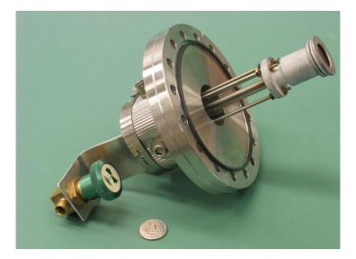
Figure 3.4: Photo of the Colutron ion source which produces stable and long-lived ions via plasma or surface ionization.
