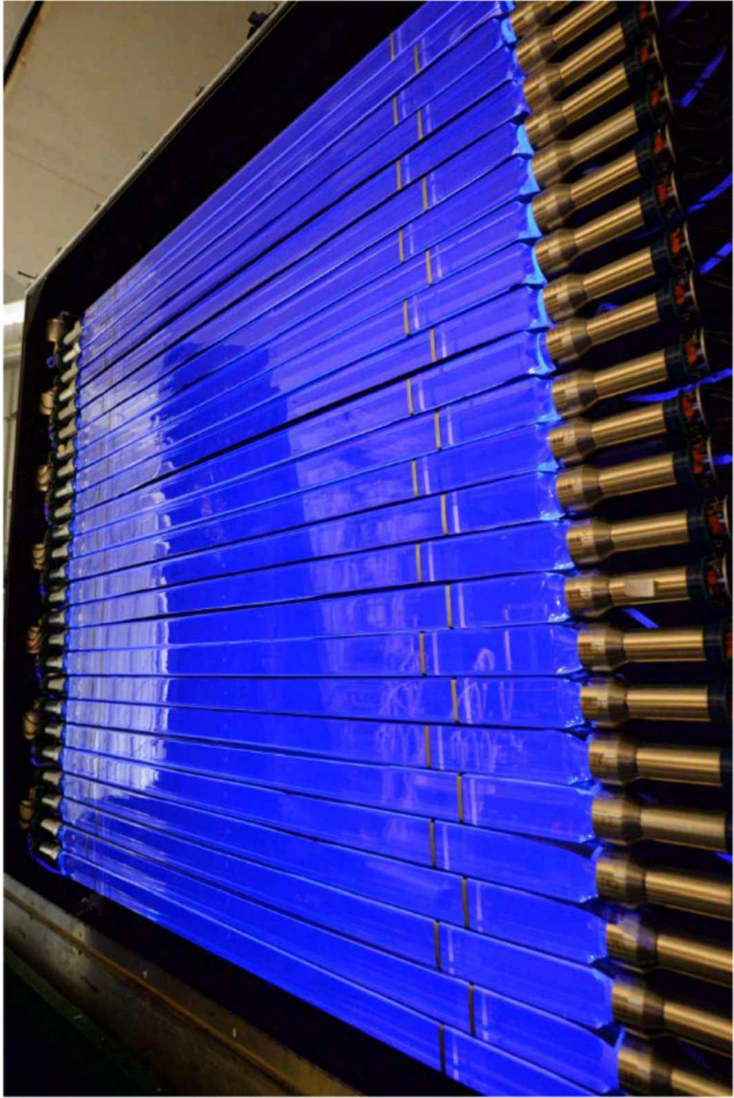
Figure 3.16: Illumination of the LANA wall through ultra violet light.
