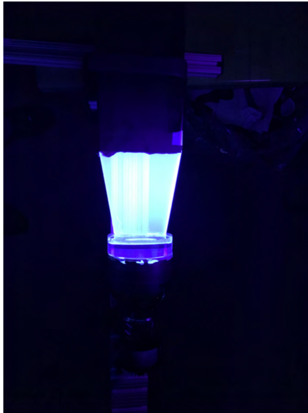
Figure 4.9: Shining UV flash light to the plastic scintillator.
