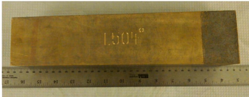
Figure 3.18: A 30 cm brass Shadow Bar to measure the background efficiency [81].
