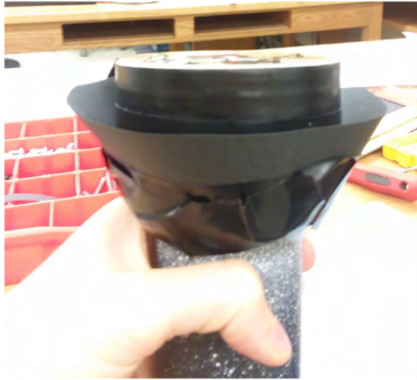
Figure 4.4: Paper ring makes umbrella like structure to hold the dripped glue.
