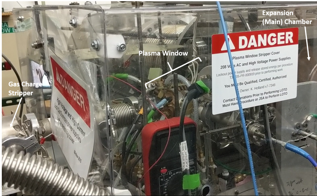
Figure 2.1: A photo of the test stand, showing the section that includes the plasma window and associated diagnostics, the gas charge stripper chamber, and the main chamber.
