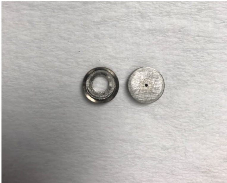
Figure 4.8: Cathode and Anticathode composed of Zr. The Zr cathodes quickly eroded over the course of the commissioning experiments. As the erosion progressed, the hole in the anticathode expanded and the cathode developed a large hole as well, which prevented operation of the PIG ion source.
