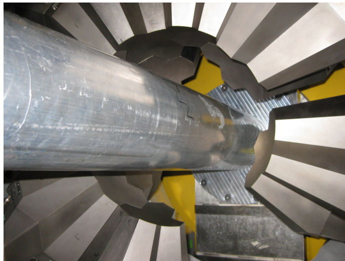
Figure 3.4: The ten HPGe detector modules of the GRETINA array directed at the secondary 188 \text{ mg/cm}^2 ^9\text{Be} target located within the six inch diameter beam line. The distance between the endcap of each detector and the target position is around 18 cm.
