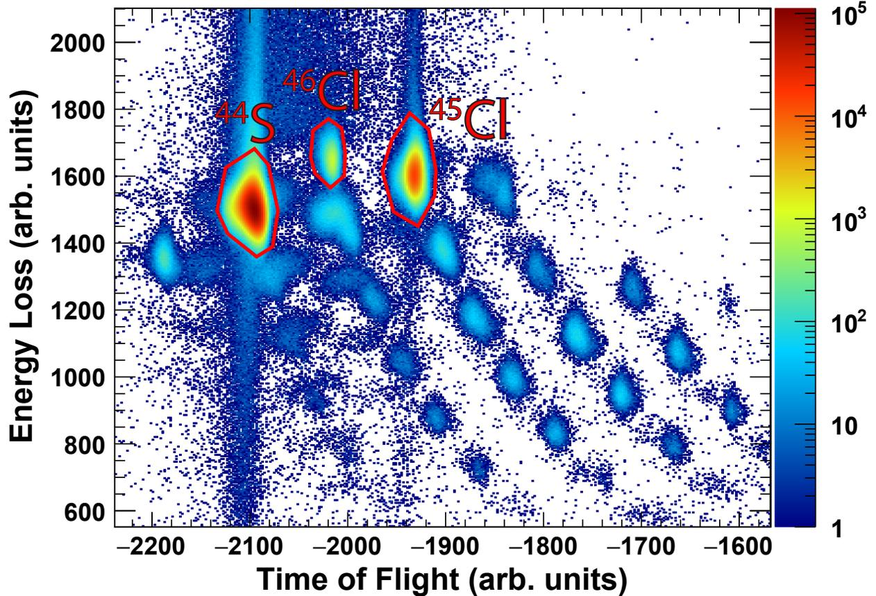
Figure 3.5: Particle identification plot utilizing energy loss and time of flight for the  $^{44}\text{S}$  setting. The energy loss is measured in the S800 ionization chamber and is proportional to  $Z^2$  and the time of flight is measured between the OBJ and E1 plastic scintillators and is proportional to  $A/Z$ .
