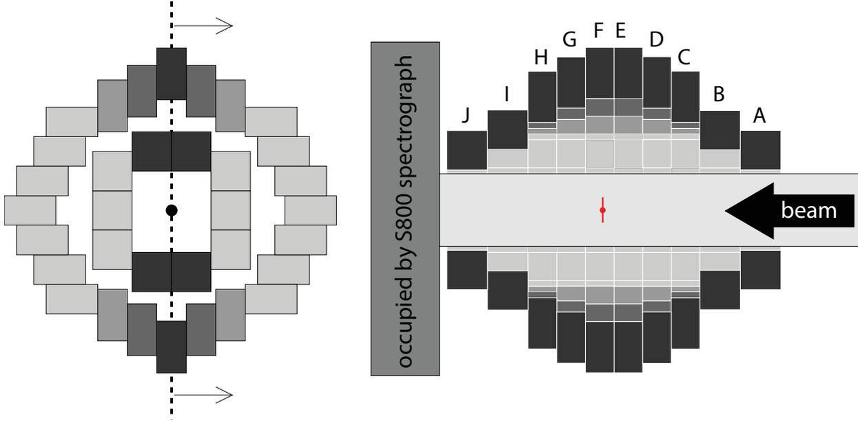
Figure 3.6: Illustration of the arrangement of CAESAR into 10 rings of detectors. Left: cross-sectional view of rings F and J perpendicular to the beam axis. Right: the  $3 \times 3 \times 3$  inch detectors occupy the two most upstream (A,B) and two most downstream (I,J) rings while the  $2 \times 2 \times 4$  inch detectors occupy the six middle rings (C-H). The target position is shown in red. Figure taken from [14].
