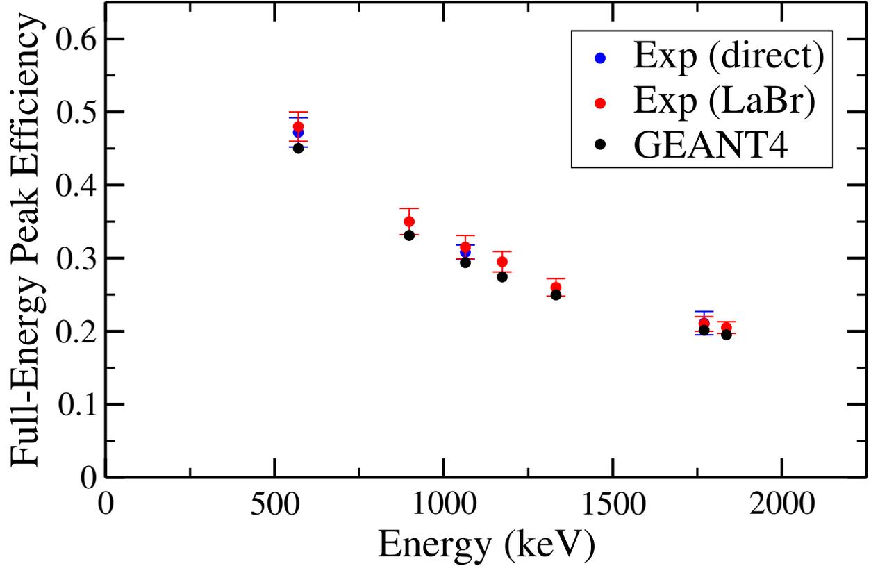
Figure 3.11: Full-energy peak efficiency of CAESAR as a function of energy as determined from direct measurement of a low-activity  $^{207}\text{Bi}$  source and from coincidence measurements with a  $\text{LaBr}_3(\text{Ce})$  detector for  $^{60}\text{Co}$ ,  $^{88}\text{Y}$ , and  $^{207}\text{Bi}$  sources compared to predictions from GEANT4 simulations. The efficiency curves here were produced treating the 192 detectors of CAESAR independently (no addback applied).
