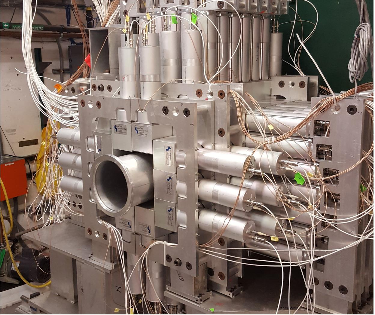
Figure 3.7: Photograph of the 192 CsI(Na) detectors composing CAESAR in front of the S800 spectrograph.
