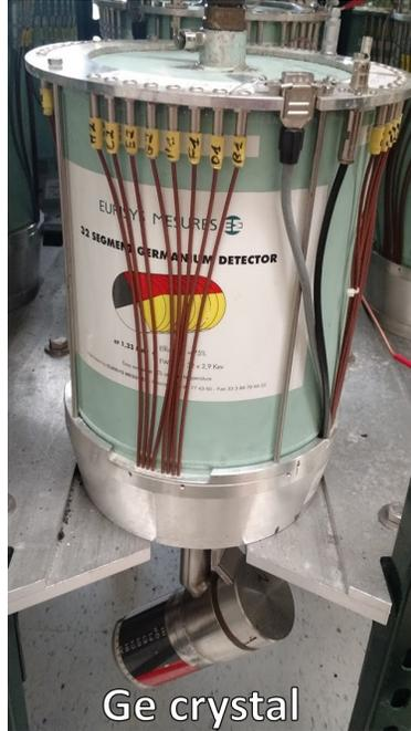
Figure 2.9: A single SeGA detector, outside of the experimental setup. The green cylinder is the liquid nitrogen dewar, with the germanium crystal at the bottom of the image. The preamplifiers are contained inside the metal casing.
