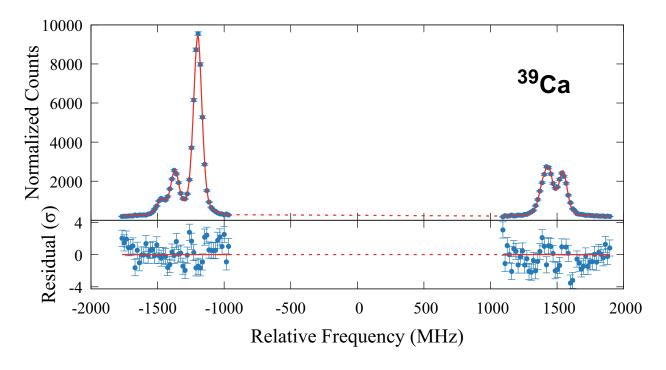
Figure 3.4: The hyperfine spectrum measured for <sup>39</sup>Ca, along with the residuals from the fit using six pseudo-Voigt functions as described in Section 3.2.
