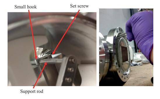
Figure A.11: Photographs showing how the elliptical reflectors are attached to the support rods. On the left the interior of the beam pipe is shown. A small "J" shaped hook holds the elliptical reflector assembly up against the support rods. It is locked in place with a set screw on the side facing out the side flange, and so it can be accessed from outside with careful use of tweezers and a long hex wrench, as shown in the photo on the right.
