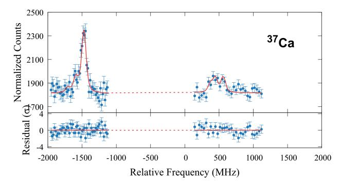
Figure 3.2: The hyperfine spectrum measured for <sup>37</sup>Ca, along with the residuals from the fit using six pseudo-Voigt functions as described in Section 3.2.
