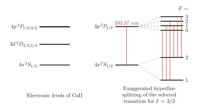
Figure 2.4: Atomic states, and hyperfine splitting. On the left, the electronic levels for Ca II are drawn [41]. On the right, the selected transition is drawn, along with the hf splitting for I = 3/2, as in  $^{37,39}$ Ca [42]. The allowed hf transitions are marked in red.
