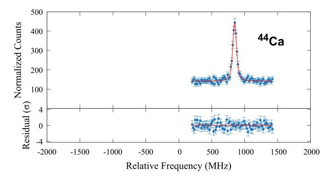
Figure 3.6: A typical spectrum measured for the calibration <sup>44</sup>Ca, along with the residuals from the fit using a pseudo-Voigt function as described in Section 3.2.
