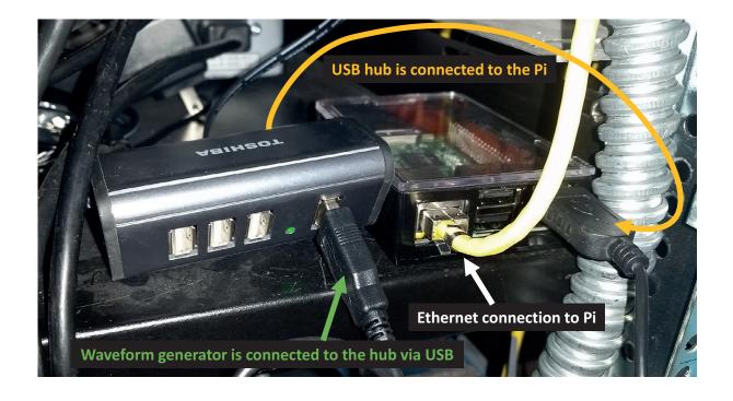
Figure A.19: Photograph of the Raspberry Pi 3B+ and its connections used to interface with the waveform generator. This is in the rack inside the high voltage cage. Rather than connect the waveform generator directly to the Pi, a USB hub must be placed in between, otherwise the Pi does not recognize the device.
