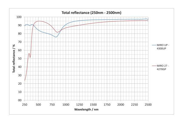
Figure A.8: Reflection data for the aluminum sheeting used for the reflective surfaces of the new PDS. The MIRO 4300UP was used, in order to allow for good reflectivity throughout the UV range  $(250-450\,\mathrm{nm})$ .
