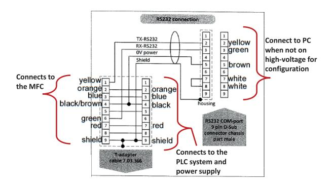
Figure A.17: Schematic showing the wiring of the custom "T" connector being used for the MFC. The diagram is taken from the manual provided by Bronkhorst, and color labels are added to indicate the actual wires used within the connector. The left side of this figure connects to the MFC, and the connection on the lower right allows for power and analog controls to be attached. The upper right connector is used for serial communication with a PC, and is not usually connected.
