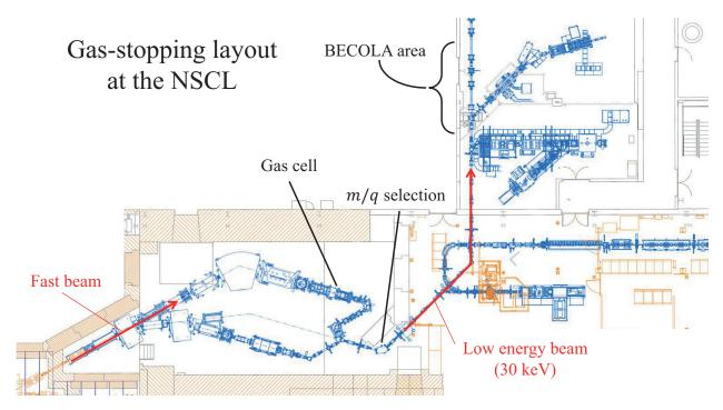
Figure 2.2: The gas stopping layout at the NSCL. Fast beams of rare isotopes are brought in from the left and are introduced to the gas cell, following a solid degrader. The ions are then thermalized in the helium buffer gas. On extraction from the gas cell, the desired charge/mass ratio can be selected using a dipole magnet. The low energy beam is then transported to the BECOLA facility, where collinear laser spectroscopy is performed.
