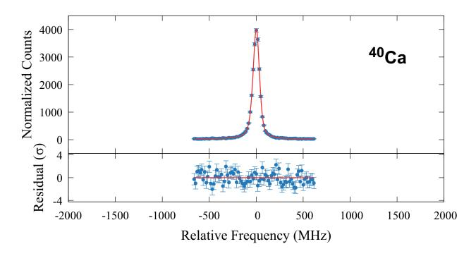
Figure 3.5: A typical spectrum measured for the reference <sup>40</sup>Ca, along with the residuals from the fit using a pseudo-Voigt function as described in Section 3.2.
