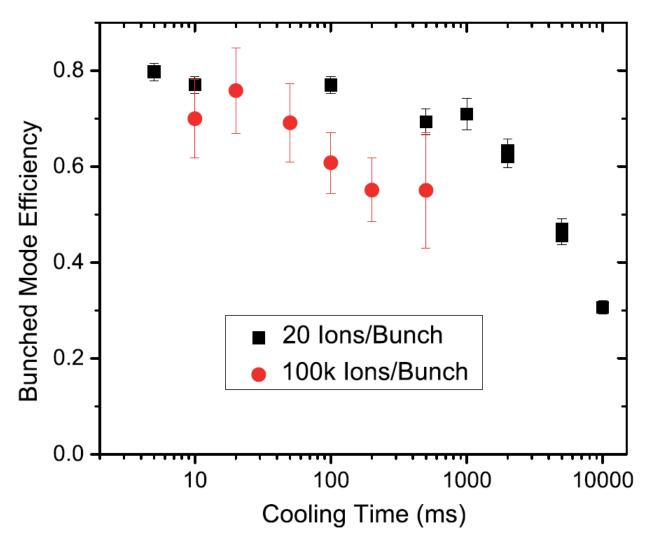
Figure 2.9: The bunching efficiency as a function of cooling time. As shown by the black squares, with small quantities of ions there is minimal reduction in efficiency for holding times up to one second. These measurements were made using potassium ions. Figure from ref. [45].
