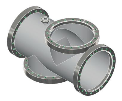
Figure A.7: A schematic of the beampipe used to enclose the two new detection regions. The 8 in flanges on the top and bottom, which are offset from one another, are the location of the two new detection regions. A small flange opposite each allows a high voltage feedthrough in order to apply the scanning potential to the detection region, as shown in Figure A.12.
