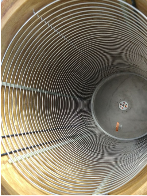
Figure 2.5: A photography of the inner volume of the AT-TPC wall with the inner rings of the field cage installed. The outer rings of the field cage have a larger diameter and one installed on the outer surface of AT-TPC cylinder. The electric field is uniform throughout the volume of the field cage thanks to the concentric ring-shaped electrodes connected by a resistor chain that gradually steps down the voltage between each ring.
