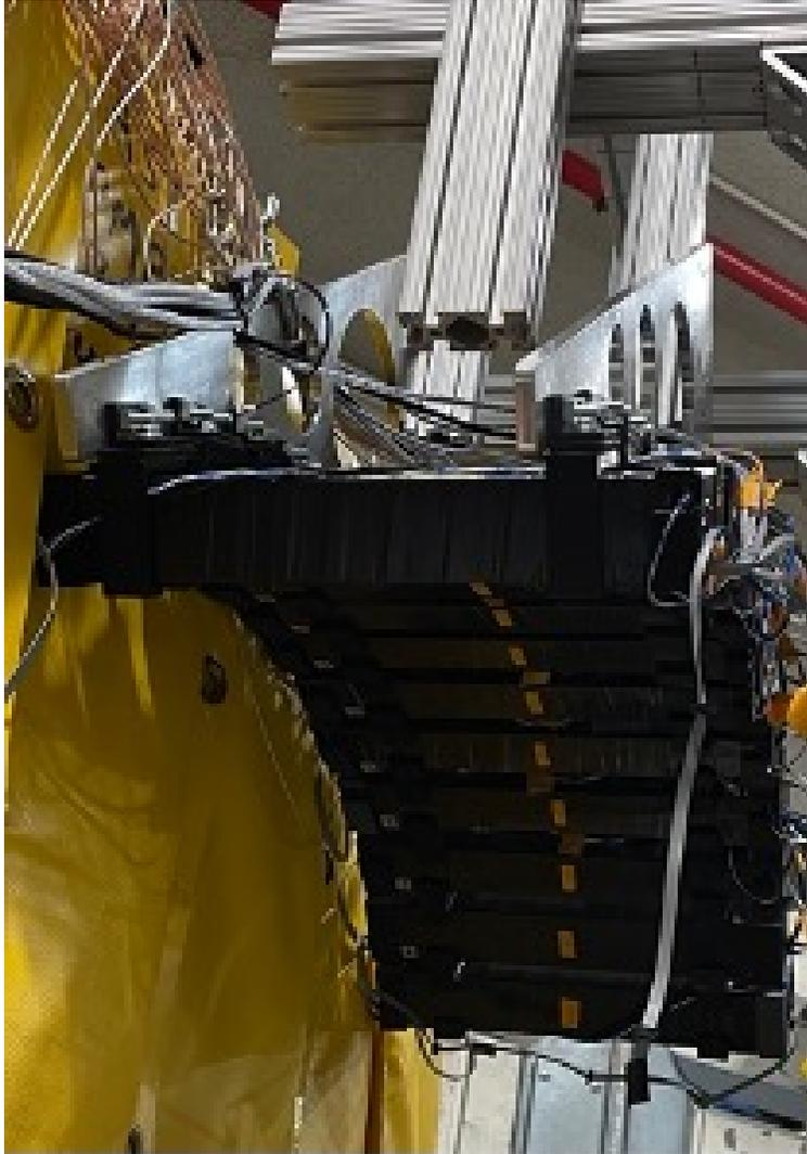
**Figure 3.13:** An array of 10 NEXT modules assembled for the experiment at Argonne National Laboratory.
