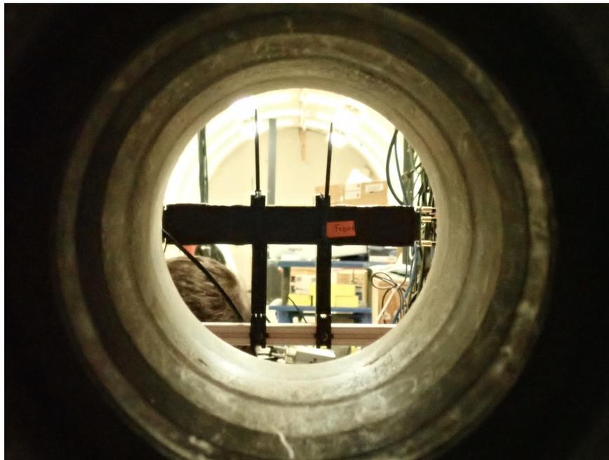
**Figure 4.2:** The experimental setup at EAL. The NEXT modules were placed at a distance of 5 m from the target assembly inside the 30 m long neutron time-of-flight tunnel. The neutron beam was collimated using concentric polyethylene collimators.
