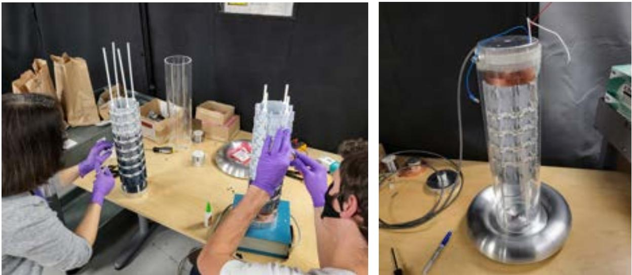
Figure 48: High voltage dividers under construction at BECOLA.
