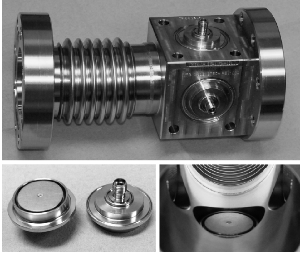
Figure 3.2: Geometry of the FRIB MEBT BPMs. The pipe radius is 23.75 mm and the pickup radius is 10 mm [6].
