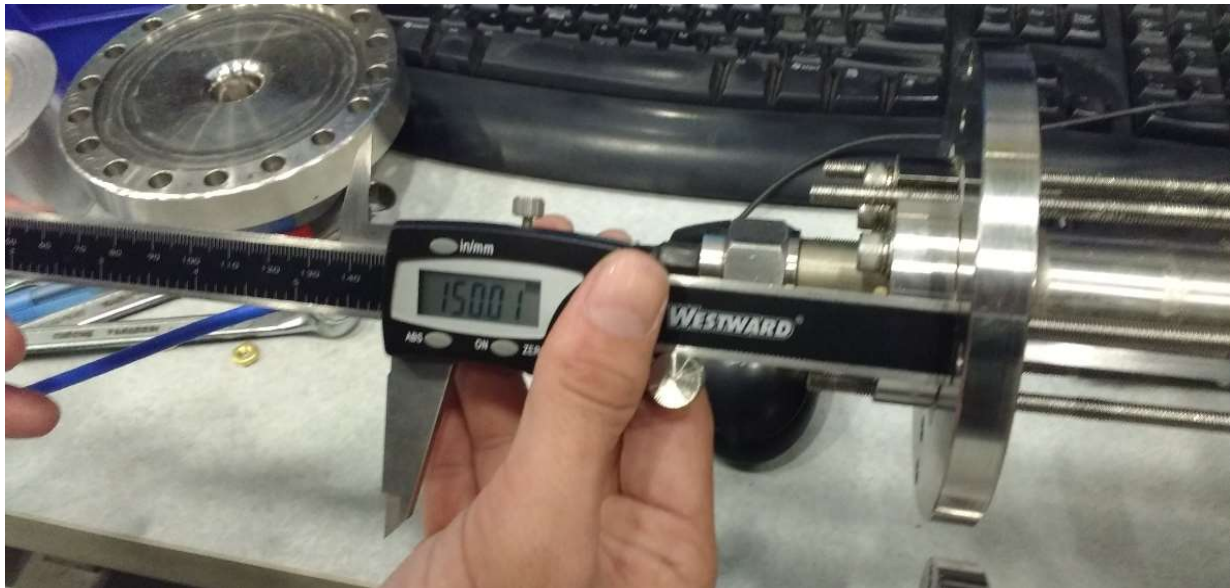
Figure 7.6: Movable coupler for 1.3 GHz cavity.
