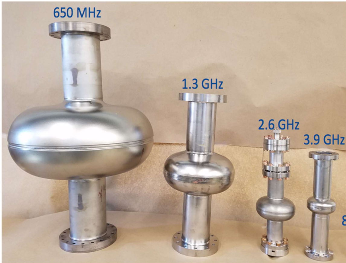
Figure 1.1: SRF elliptical cavities for different frequencies. Image Credit: Martina Martinello, Fermilab.
