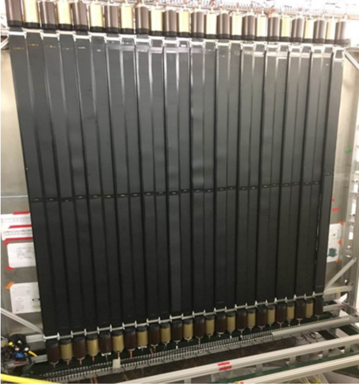
Figure 3.5: Western Michigan University Neutron Veto Wall This figure shows the Veto Wall set up in front of the LANA neutron wall stack.
