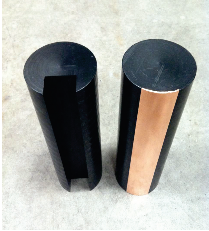
Figure 4.4: Dielectric samples with different types of anomalies. The left sample contains a 1.75-inch-wide and 1-inch-deep axial defect. The second sample contains a 2-inch-wide piece of copper tape along its main axis.
