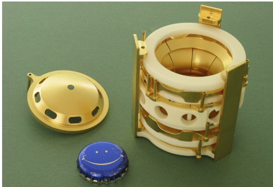
Figure 3.6. Photograph of the LEBIT Penning trap with one endcap electrode removed, from [143]. Note the hole in the endcap electrode for ion injection/ejection, and the bottle cap for scale.
