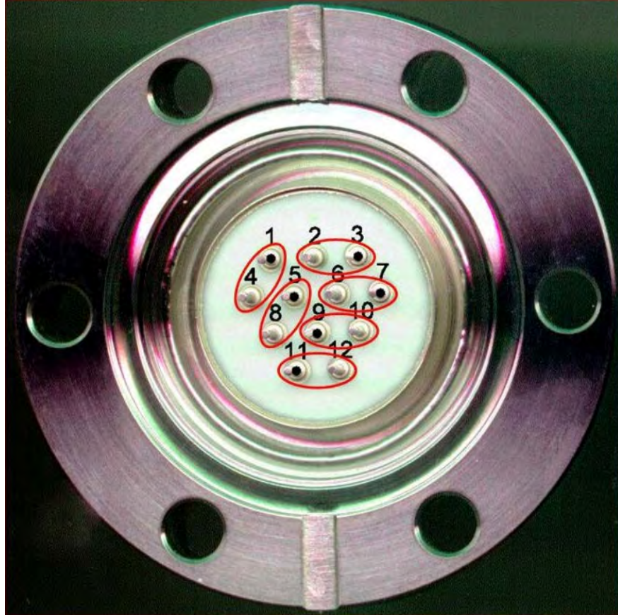
Figure A.3: Pinout for the vacuum side of the FT12TP. On the air side the pin numbers will be mirrored (e.g. top left pin is #3). Red ovals mark the pins for twisted cable pairs
