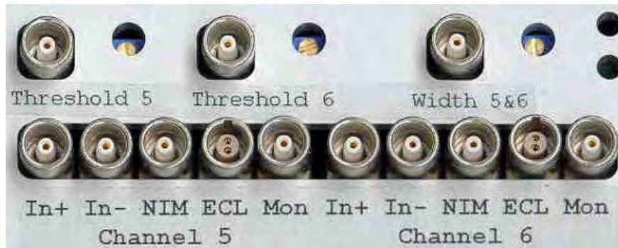
Figure A.5: The ATR19 constant fraction discriminator front panel. Two channels of six are shown.
