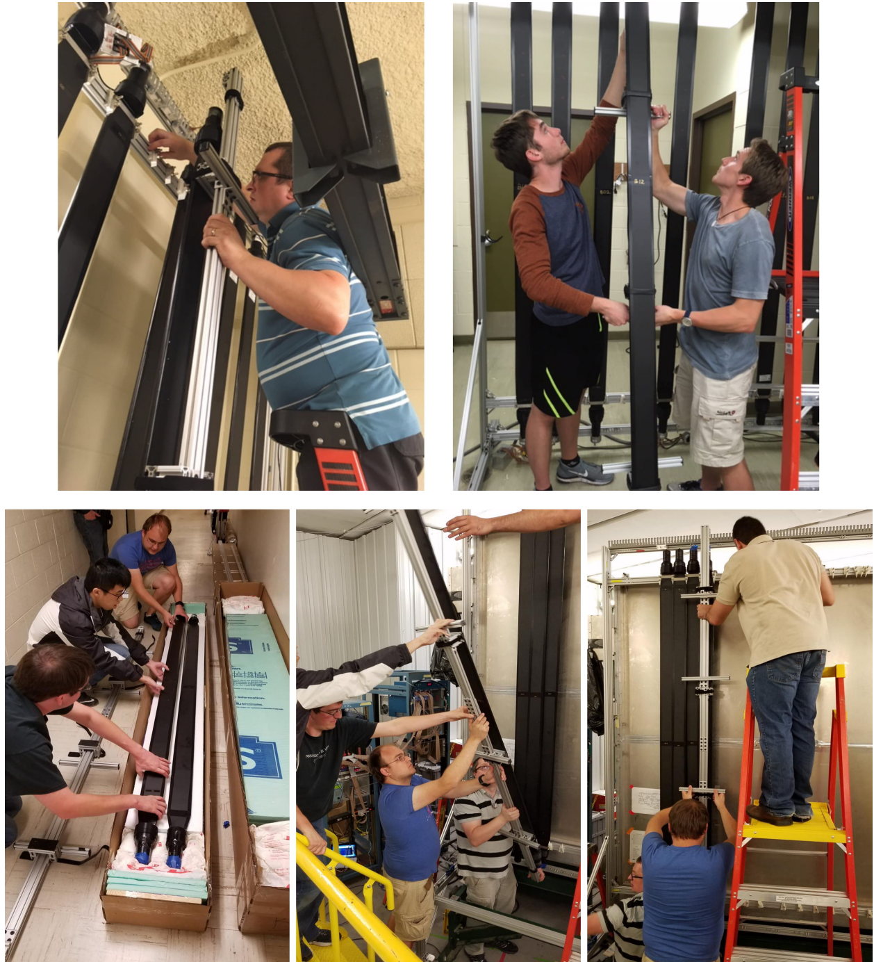
Figure 2.21: (top left panel) Professor Chajeki is testing the Charged-Particle Veto Wall frame. (top right panel) Undergraduate students from Western Michigan University and Michigan State University are moving Veto Wall bar. (bottom left panel) Veto Wall bars are being taken out from shipment packages. (bottom middle and right panel) NSCL and WMU researchers are installing the Charged-Particle Veto Wall in front of LANA.
