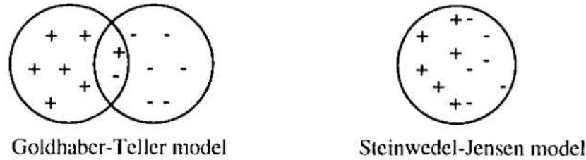
Figure 2.1 Schematic representation of giant dipole resonance in the Goldhaber-Teller model and the Steinwedel-Jensen model.
