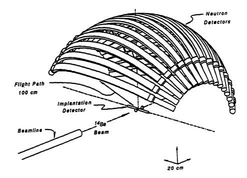
Figure 2.2 Schematic of NSCL neutron detector array [Ha91].
