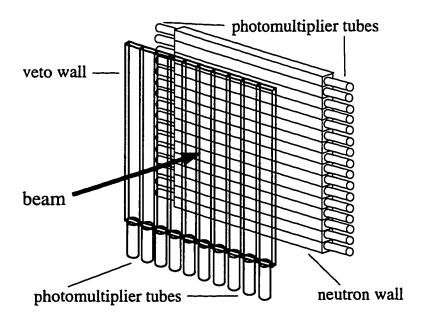
Figure 4.7 Diagram showing the geometry of the neutron and veto walls; it is not drawn to scale.
