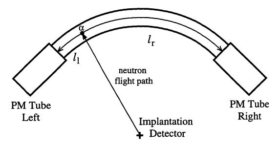
Figure 3.5 Schematic showing the geometry of a typical neutron decay. The symbol "PM" is an abbreviation for photomultiplier. Note that the diagram is not drawn to scale.
