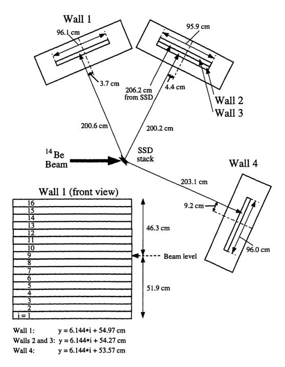
Figure 4.8 Schematic of the neutron detectors, as seen from above, showing the dimensions, geometry, and distance of these detectors from the SSD stack. A front view of neutron wall 1 is shown in the lower left corner (the geometries of the other walls are similar). The equations give the vertical position corresponding to each neutron bar i for each of the walls.
