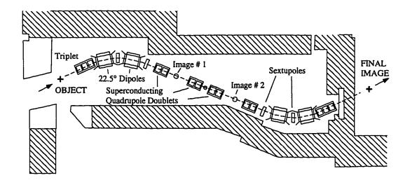
Figure 2.1 Diagram of A1200 Beam Analysis Device [Sh91].
