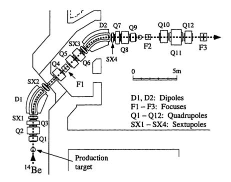
Figure 4.1 Diagram of the RIPS radioactive beam facility.
