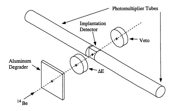
Figure 2.3 Diagram of the hardware located at the center of the NSCL array [Ha91].
