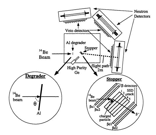
Figure 4.2 Schematic of experimental setup viewed from above with enlarged detail of the stopper (implantation detector) and the aluminum degrader. This figure is not drawn to scale, and it was, in part, obtained from [Ki93].
