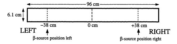
Figure 4.9 Diagram showing the geometry of a scintillator bar (as the beam sees it) and the locations of the  $\beta$  source used in the horizontal calibration.
