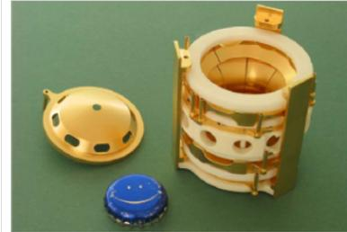
Figure 2.10: (Left) A schematic overview of the LEBIT facility. (Right) The LEBIT high-precision Penning trap with its end-cap removed. A bottle cap is shown with the trap for scale [41].
