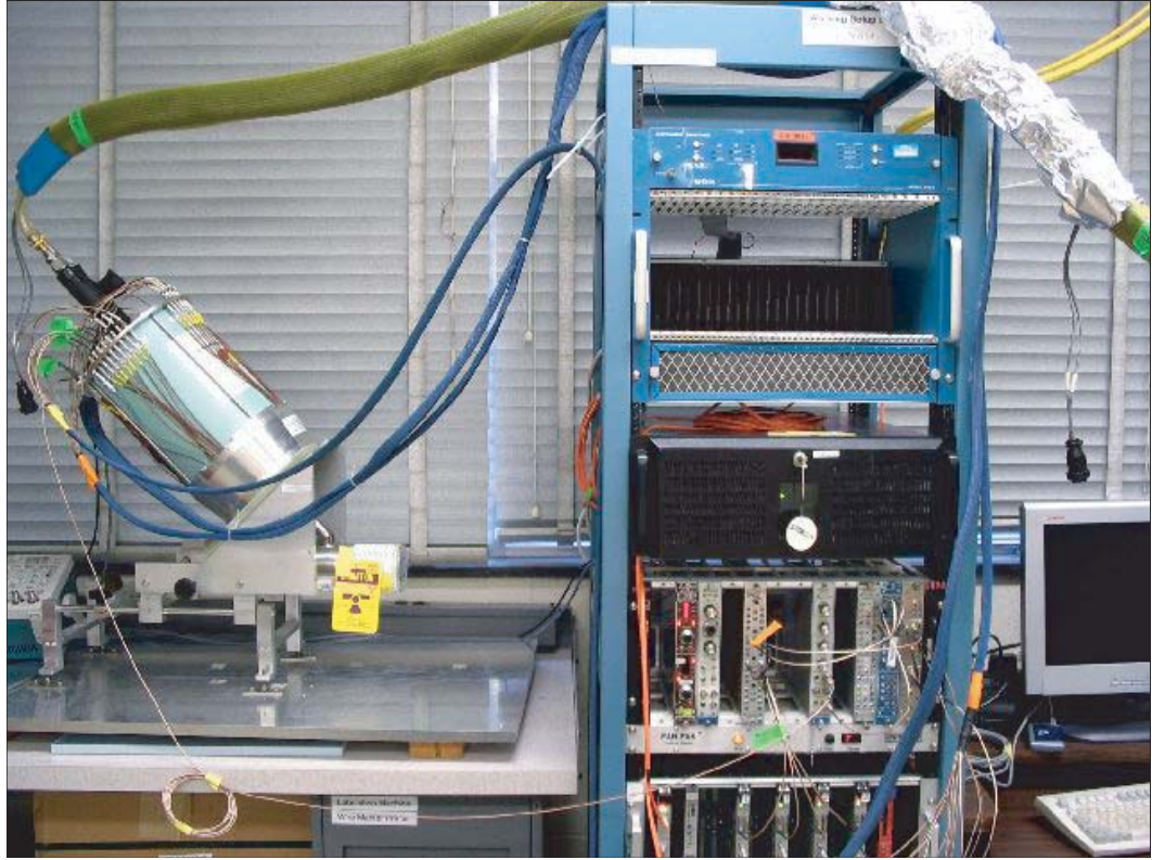
Figure 3.8: Experimental setup of the SeGA scanning stand.
