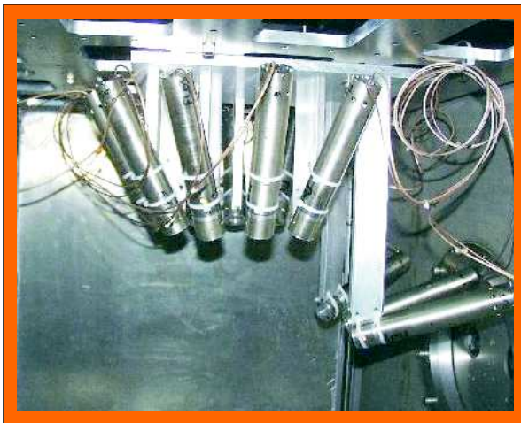
Figure 2.4: The direction of the beam is from left to right in both panels. Left: Photo of the CsI array. The most forward detector was removed during the experiment. Right: Top view of the CsI array. The CsI detectors are depicted as green cylinders.
