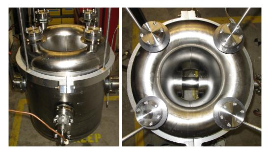
Figure 4.8: Prototype  $\beta = 0.53$  HWR manufactured and tested at MSU.
