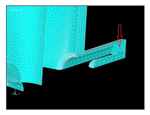
Figure 3.22: The coupler probe can be seen in the foreground connected to the RF port by the surface indicated by the red arrow. This is a quarter of the geometry cut on the symmetry planes.
