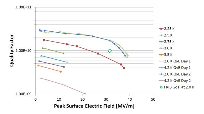
Figure 4.12: Cavity Quality Factor  $(Q_0)$  plotted versus Peak Surface Electric Field for both testing days.
