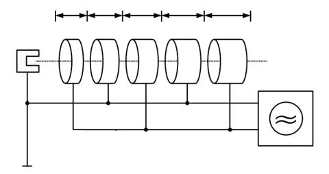
Figure 1.2: Schematic of an RF accelerator with particle source (left), voltage source (bottom right), and repeating drift tubes/gaps for acceleration. Note the increased length of the drift tubes as the particles gain energy.
