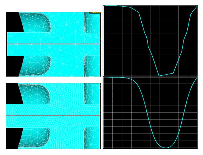
Figure 3.7: Top Left: Poorly meshed cavity, beam axis marked in red. Top Right: Resulting accelerating electric field. Note the non-physical roughness that results from the large element size. Bottom Left: Cavity with improved meshing on beam axis which is marked in red. Bottom Right: Resulting accelerating electric field. Note the improved field profile that results. Images generated in ANSYS.
