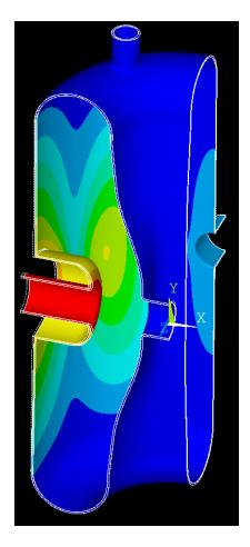
Figure 3.32: Simulation of cavity deformation for an applied tuning force.
