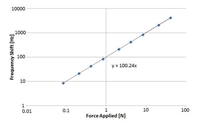
Figure 3.29: Frequency shift versus applied pressure for a mechanical simulation. Note the linearity down to very small frequency shifts.
