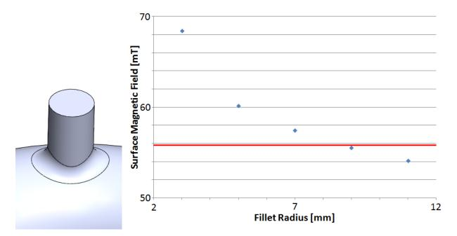
Figure 3.25: Left: Rinse port on a HWR short plate with fillet. Right: Plot of surface magnetic field on the rinse port versus radius of the fillet. The red line indicates the peak surface magnetic field in the rest of the cavity.
