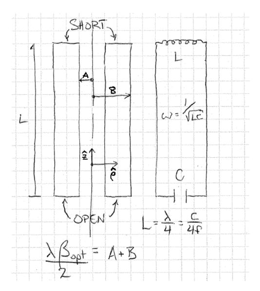
Figure 2.8: Schematic of the ideal QWR.
