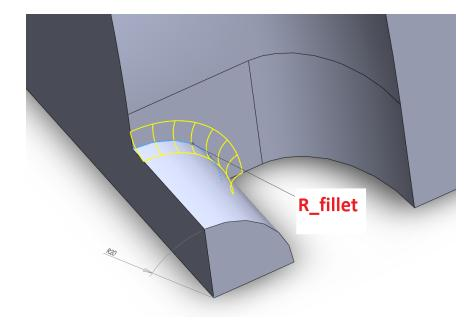
Figure 3.15: After the addition of the drift tube, a fillet is introduced to reduce the field enhancement on the inner conductor. Three symmetric planes assumed.
