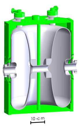
Figure 4.1: Prototype  $\beta = 0.53$  HWR manufactured and tested at MSU with helium vessel.
