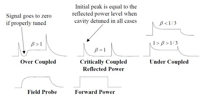
Figure 4.6: Transient behavior of the reverse power for different coupling strengths. All curves are in response to the shown forward power behavior. Image credit to Tom Powers, TJNAF.
