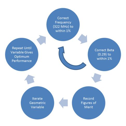
Figure 3.17: The work flow for optimization of a geometric variable.
