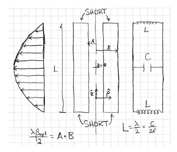
Figure 2.12: Schematic of an ideal HWR.
