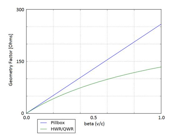
Figure 2.13: Geometry Factor plotted versus  $\beta$  for the ideal cavity geometries.
