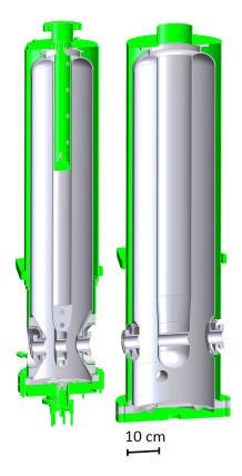
Figure 2.11: FRIB Quarter Wave Resonator designs.
