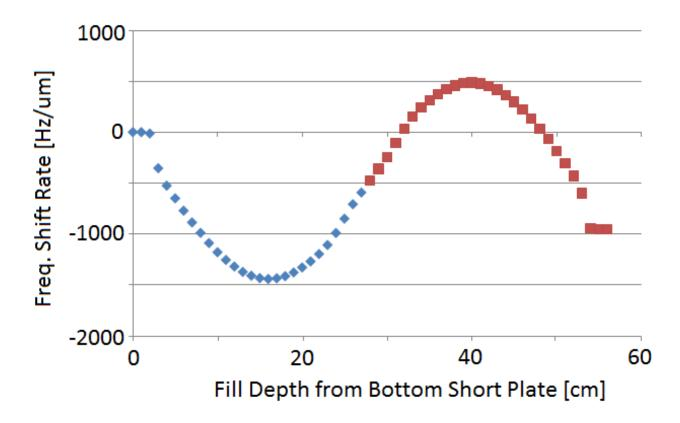
Figure 3.26: Plot of simulated etching coefficient for a prototype  $\beta = 0.53$  HWR filled with acid to different levels. The blue diamonds represent simulation data, and the red squares are this data mirrored assuming symmetry.
