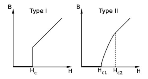
Figure 2.14: Magnetic field just inside superconducting material around transition for Type 1 and 2 materials. Note the sudden penetration for Type 1 and the gradual break down for Type 2.
