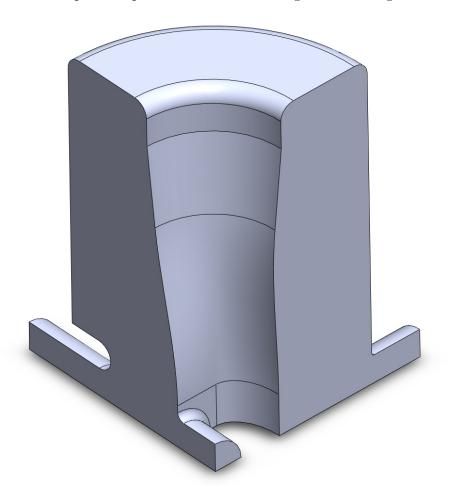
Figure 3.11: HWR vacuum space cut on three symmetry planes.
