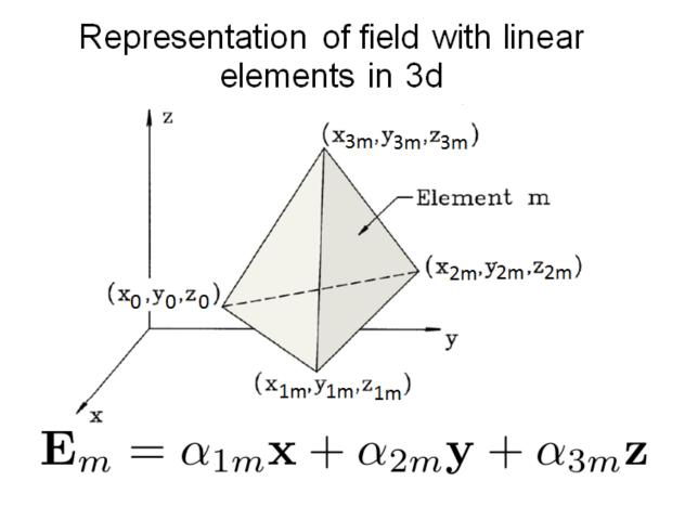
Figure 3.2: Structure of a first order (linear) tetrahedral element. Image credit to F. Krawczyk.
