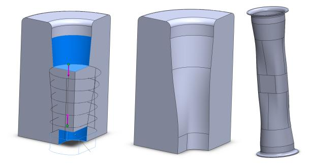
Figure 3.14: Left: Setup for the loft cut to complete the inner conductor shape. Automatic spline guide curves for the cut can be seen in black with the tangential boundary condition shown by purple arrows. Center: Resulting inner conductor shape with smooth transition between magnetic and electric field regions. Three symmetric planes assumed. Right: Resulting inner conductor geometry.
