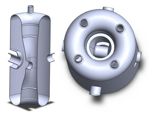
Figure 3.33: Left: Stiffening ring added to the inner conductor in section view. Right: Top down view of the stiffening ring with full cavity.
