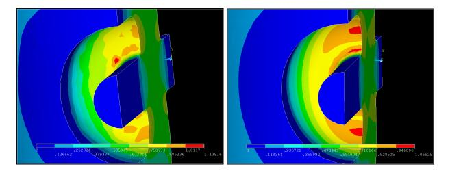
Figure 3.8: Left: Magnitude of the surface electric field on a beam port cup with inadequate meshing for surface field accuracy. Right: Identical geometry with improved meshing and more realistic surface fields.
