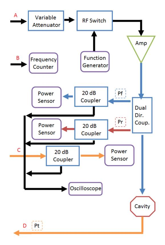
Figure 4.14: One half of the RF circuit for a phase lock loop for cavity testing (circulator, isolators, and RF diodes excluded). Letters in Red connect to the other half of the RF circuit, seen on the previous page.
