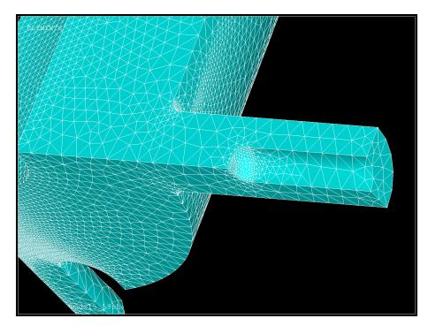
Figure 3.1: A cavity vacuum space meshed with tetrahedral elements, a coupler probe is in the foreground with a beam port cup visible in the background.
