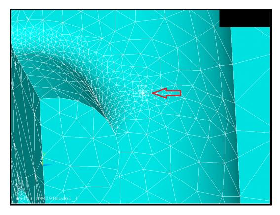
Figure 3.6: The intersection of four surfaces can force excess mesh density, indicated by the red arrow. Images generated using ANSYS.
