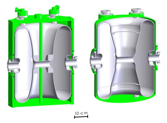
Figure 4.9: Left: Mechanical design of the prototype  $\beta = 0.53$  HWR, manufactured and tested at MSU. Right: More recent mechanical design of a  $\beta = 0.53$  HWR that shares many design features with the HWR designed in this document.
