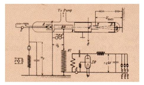
Figure 1.3: Schematic of Wideroe's Demonstration Accelerator
