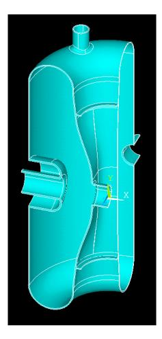
Figure 3.27: Material space after importation into ANSYS-APDL.
