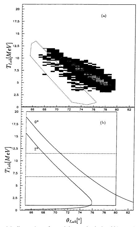
Figure 8.5: Comparison of actual data and calculated kinematics. (a) The collected proton scattering data displayed on the same scale as the calculated kinematics in (b). The dashed box indicates the identified inelastic events. (b) Calculated kinematic curves of energy as a function of scattering angle in the laboratory frame. The solid box shows the field of view of the telescopes. The dashed lines show the punch through energies for a proton penetrating into the next stage of the telescope.
