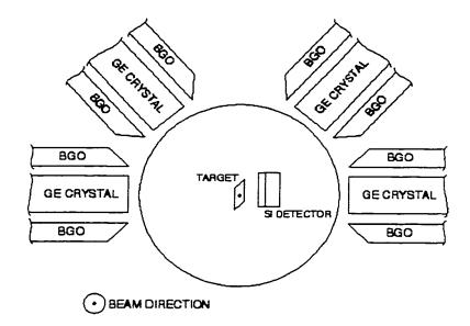
Figure 3.1: Schematic of the  ${}^{196}Pt(p, p'\gamma)$  experimental apparatus.
