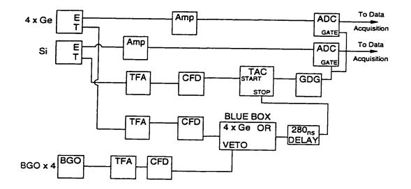
Figure 3.3: Diagram of the electronics. Both the signal and logic electronics are included.
