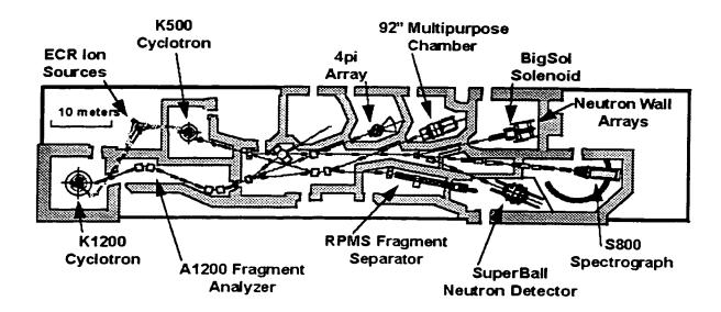
Figure 7.1: The layout of the NSCL experimental facility. The figure shows the K1200 cyclotron where the primary beam is accelerated, the A1200 mass fragment separator for production and selection of the radioactive secondary beam, and the S2 experimental vault at the tail end of the RPMS fragment separator where the  $p(^{20}O,p)^{20}O$  scattering experiment was performed.
