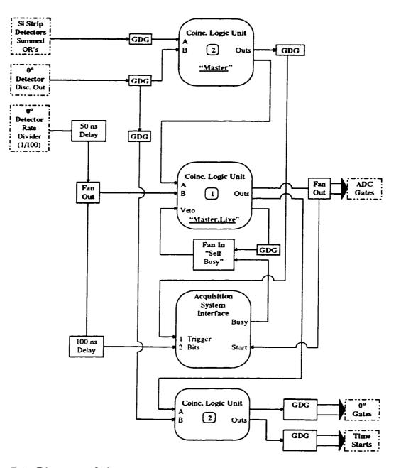
Figure 7.8: Diagram of the master electronics which generated event triggers and gates. The boxed number in the coincidence logic units indicates the coincidence level required between the two inputs labeled A and B.
