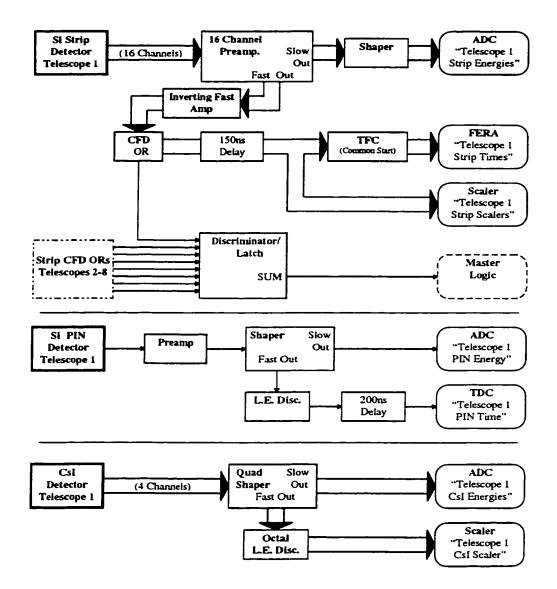
Figure 7.7: Electronics diagram for a single particle telescope. Gates and time starts were generated by the master electronics shown in Figure 7.8 and are not included explicitly here.
