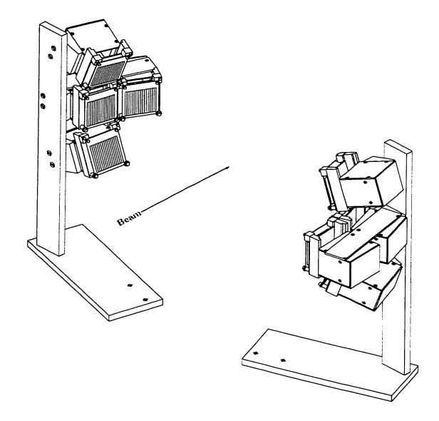
Figure 7.5: Positioning of the FSU-MSU charged particle telescope array. Each telescope is a three stage detector consisting of a position sensitive Si strip detector, a PIN diode, and a CsI scintillator. Telescopes 1,2 and 3, on the left side, are centered at 75° with respect to the beam axis, and telescope 4 is at 60.5°. On the right, telescopes 5,6 and 7 are centered at 70°, and telescope 8 is at 84.5°.
