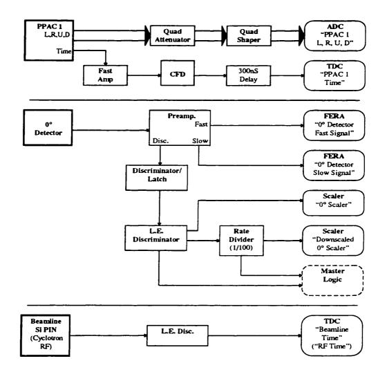
Figure 7.6: Electronics diagram for the beam detectors. Electronics for PPACs 1 and 2 were identical. Gates and time starts were generated by the master electronics shown in Figure 7.8 and are not included explicitly here.
