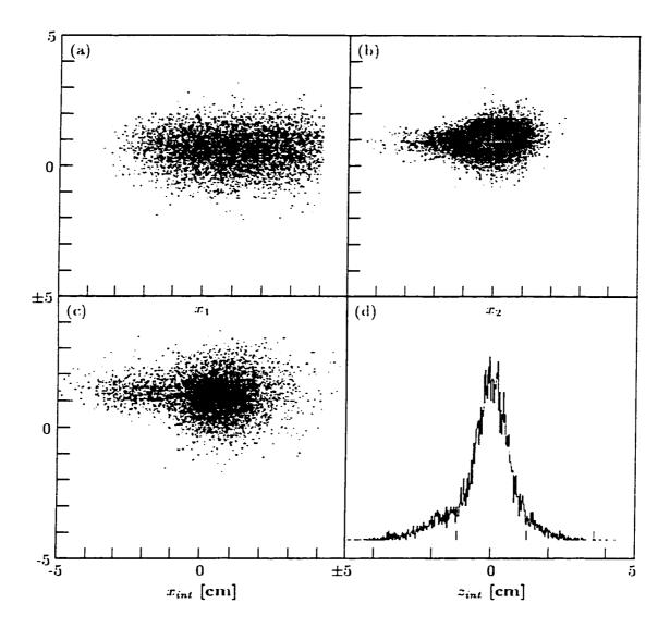
Figure 8.2: Examples of beam tracking spectra show two dimensional position spectra for the beam measured at (a) PPAC 1 and (b) PPAC 2, (c) the projected transverse position, and (d) the z position spectra on target.
