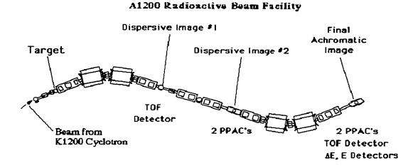
Figure 7.2: A1200 mass fragment separator at the NSCL. The A1200 is used to identify and select secondary beams after fragmentation of the primary beam.
