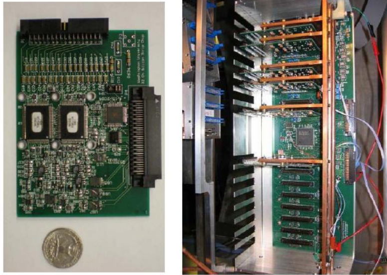
Figure 3.18: (Left) Photograph of a chipboard with two ASIC's attached. A U.S. quarter is used for size reference. (Right) Photograph of a motherboard with 6 chipboards inserted.
