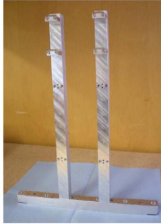
Figure 3.29: A photograph of reference posts used for transforming different laser positions.
