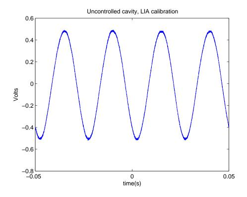
Figure 8.4. Cavity phase measurement with Lock-in-Amplifier at 18°.
