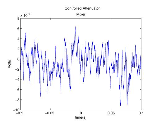
Figure 8.9. Phase error of controlled Attenuator equates to 0.054°.
