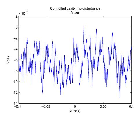
Figure 8.7. Controlled cavity with no disturbance resulting in 0.045° error.
