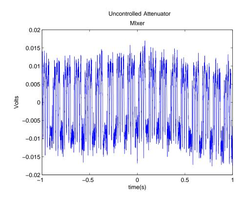
Figure 8.8. Phase error of uncontrolled attenuator equates  $0.1198^{\circ}$ .
