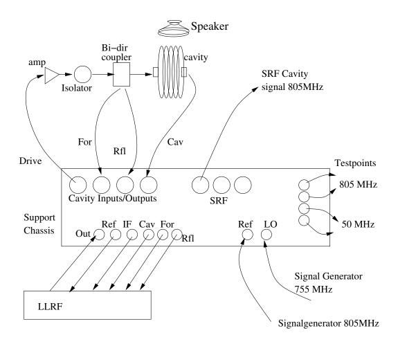
Figure 8.1. Test set-up for support chassis.
