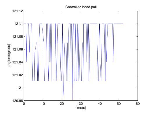
Figure 8.3. 0.12° phase disturbance from a controlled bead pull.
