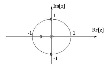
Figure 5.4. Example z-plane plot of H(z).
