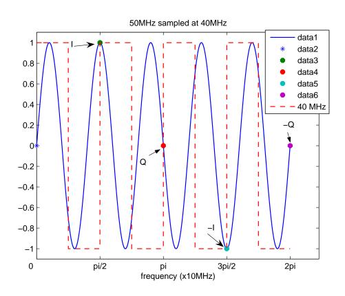
Figure 4.6. Sampling 50 MHz signal with a 40MSPs ADC.
