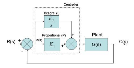
Figure 5.3. Block diagram of a PI compensator.
