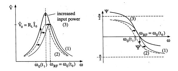
Figure 2.9. Effects of disturbance on resonant frequency.
