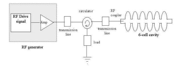
Figure 2.1. General system set-up for a single 6-cell elliptical cavity.
