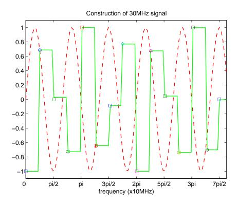
Figure 5.11. DAC output with additional points from 'afterburner'.
