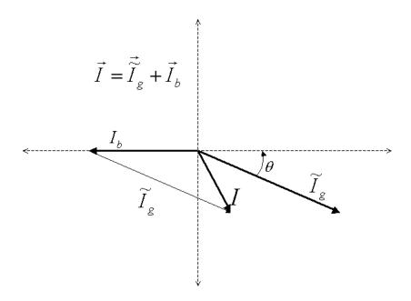
Figure 2.8. *I* representing generater and beam currents
