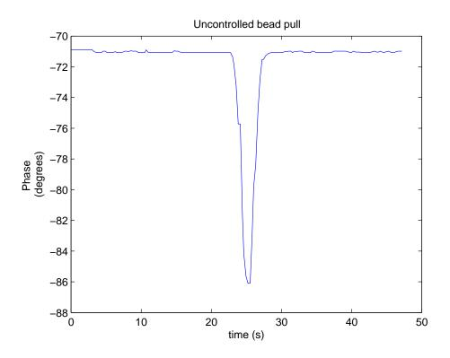
Figure 8.2. 15.1° phase disturbance from an uncontrolled bead pull.
