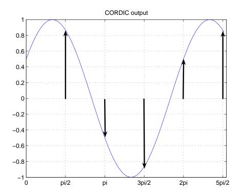
Figure 5.5. Simulated plot of CORDIC output.
