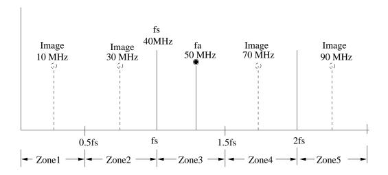
Figure 4.5. Example of images from a 50 MHz signal sampled at 40 MHz.
