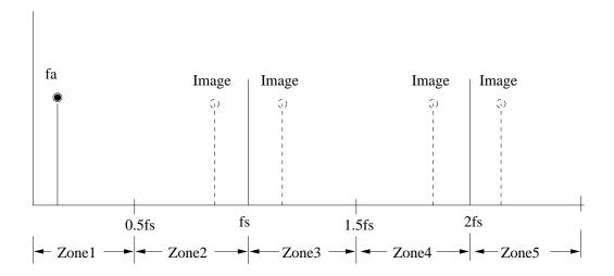
Figure 4.1. Signal  $f_a$  sampled at  $f_s$  using ideal sampler with images at  $|\pm mf_s \pm f_a|$ , m = 1, 2, 3, ...
