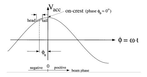
Figure 2.6. Phase, i. e. synchronous phase  $\phi_s = \phi_b$ .
