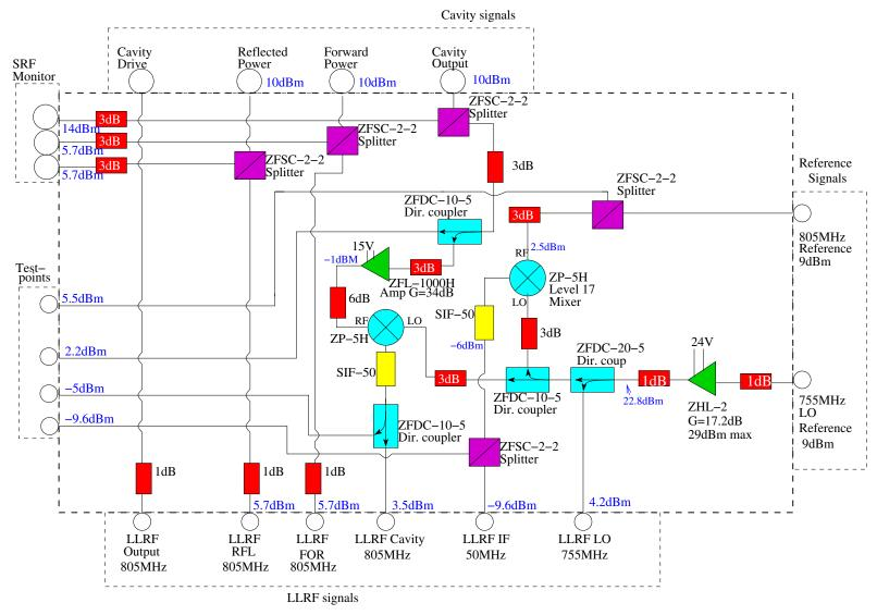
Figure 6.4. LLRF Support chassis schematic.
