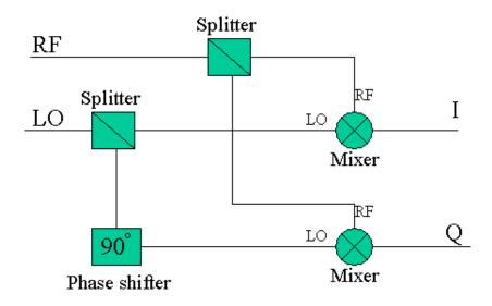
Figure 4.4. Analog method of determining I and Q values.
