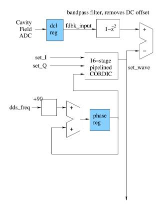
Figure 5.7. Set-point creation by DDS and Cordic.
