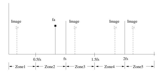
Figure 4.2. Sampling a signal outside the first Nyquist zone, image falls within the first Nyquist zone.
