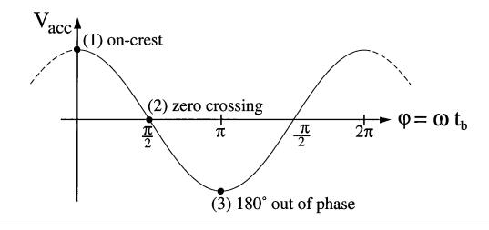
Figure 2.5. Timing of the bunch.
