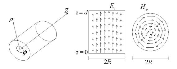
Figure 2.4. Cavity fields for  $TM_{010}$ .
