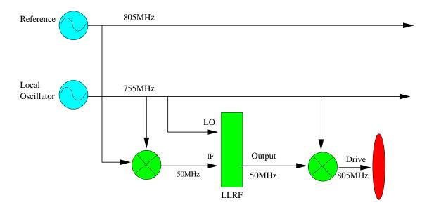
Figure 6.2. Mixer downconversion and upconversion using noisy reference.
