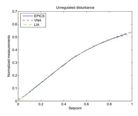
Figure 8.11. Amplitude measurements vs. set-point, uncontrolled with a disturbance.
