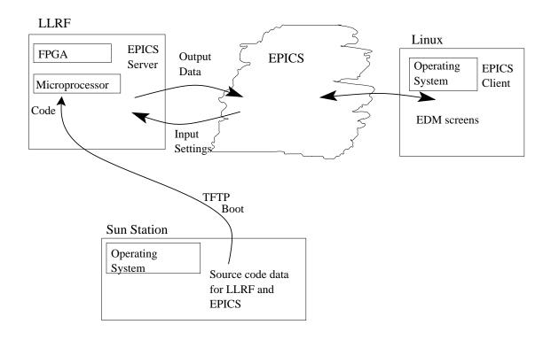
Figure 7.1. Relationship between hardware components.
