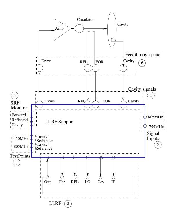
Figure 6.3. LLRF support chassis block diagram.
