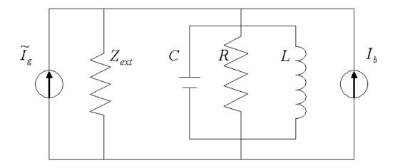
Figure 2.7. Equivalent RLC circuit with load.
