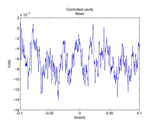
Figure 8.6. Controlled cavity mixer error measurement of 0.0526°.
