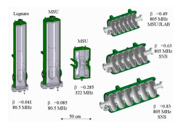
Figure 1.1. Illustration of various linac cavities.
