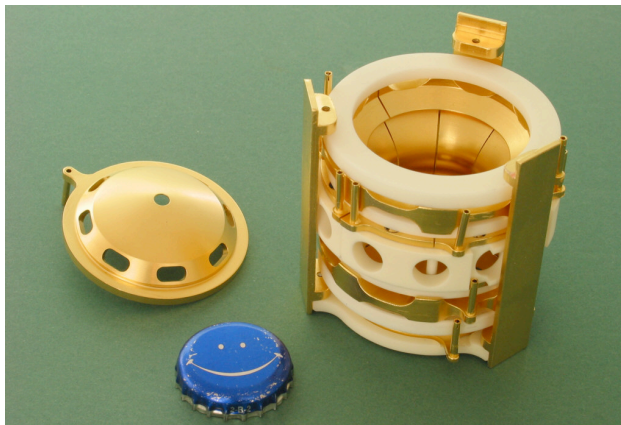
Figure 3.10. The LEBIT high-precision Penning trap with one endcap electrode removed. Note the hole in the endcap for ion injection/ejection.
