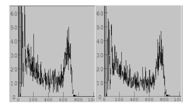
**Figures I.12a and I.12b**: Individial pad pulse spectrum for CRDC pad #86 before and after gain matching. Note the position of the peak has increased along the X-axis to match the pad with the other pads.
