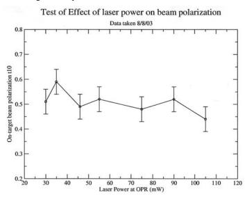
Figure III.12: On-target beam polarization vs. laser power.
