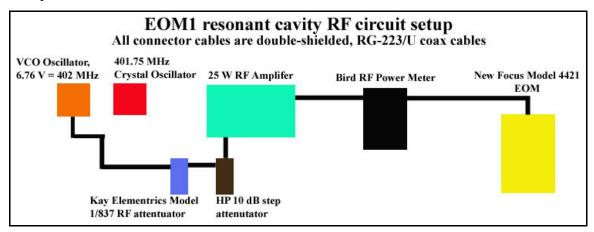
Figure III.9: Electronics setup for new EOM1
