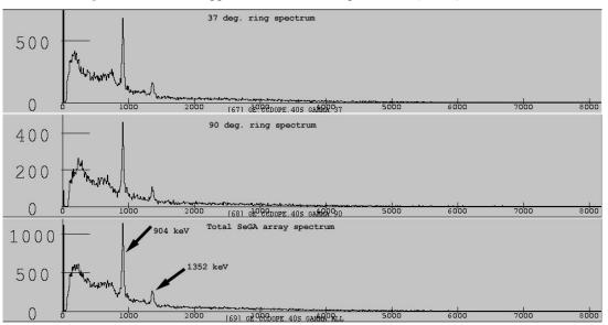
**Figure I.16b**: Doppler Corrected spectra for  $d({}^{42}S, {}^{40}S)X$  with Beta=0.417. Note the alignment of the peaks in the two detector rings.
