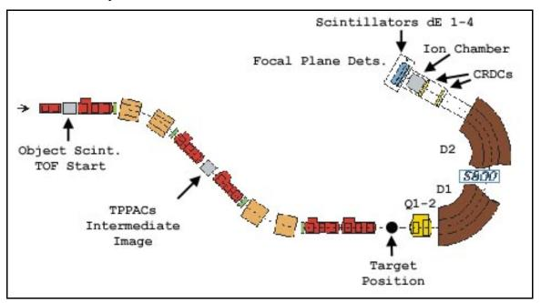
Figure I.6: Setup of the S800 spectrograph. The liquid deuterium target and the SeGA array are placed at the target position.
