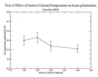
Figure III.11: On-target beam polarization vs. ionizer current for the first test experiment.
