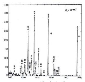
**Figure I.2a**: Spectrum of states populated in the  ${}^{48}Ca({}^{7}Li, {}^{6}He){}^{49}Sc$  reaction [6]. The single particle states are represented by the large peaks in the spectrum.
