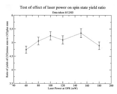
Figure III.14: Ratio of yields of spin states vs. laser power. The polarization ratio was measured to be higher with 150mW vs. the initial 60 mW of laser power.
