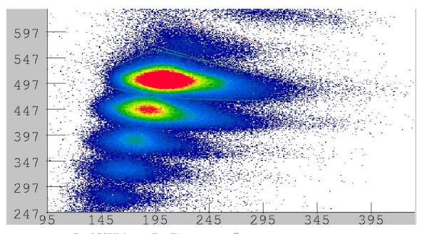
**Figure I.20**:  $\Delta E - ICSUM$  vs.  $\Delta E - E1$  gated on the <sup>40</sup>S beam. The energy loss of the sulfur blob in the spectrum is identified in the ion chamber with the beam elastic scattering run. The blobs from top to bottom represent events from chlorine, sulfur, phosphorus, and so on.
