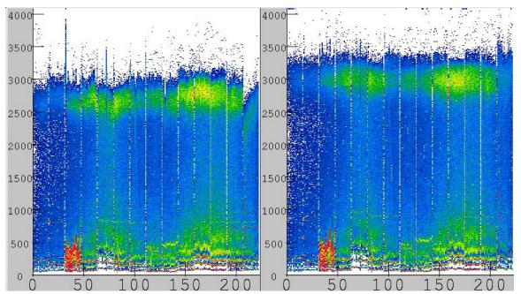
Figures I.11a and I.11b: CRDC1 pad summary spectrum before (left panel) and after gain matching (right panel). Pulses from calcium events are shown by the upper green areas. "Badpads" are shown as the white gaps between groups of pads.
