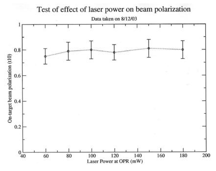
**Figure III.13**: On-target polarization vs. laser power on 8/12/03 with the retro-reflecting mirror (concave mirror with hole) removed. The result shown was obtained by passing the laser through the atomic beam and a single reflection back through.
