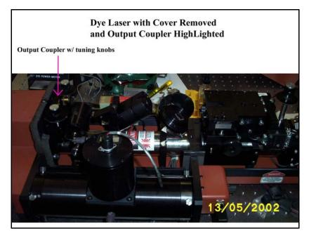
Figure A.IV.1: Dye laser output coupler.
