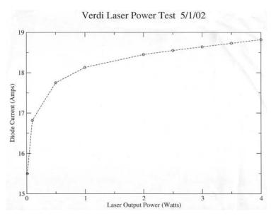
**Figure III.6:** Laser diode current vs. laser power output for the Verdi V-5 laser. The dashed line between points is to guide the eye. Deviations from this curve may signal that the laser diode is deteriorating.
