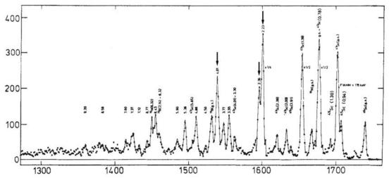
**Figure I.2b**: Spectrum of states populated in the  ${}^{50}Ti(d, {}^{3}He){}^{49}Sc$  reaction [5]. The strong single nucleon hole states at 2.23 MeV, 2.36 MeV and 4.01 MeV are shown with arrows. The large peaks at the low energy end (right side) of the spectrum were due to contaminants.
