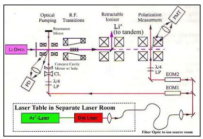
**Figure III.2**: Optics Setup for OPPLIS prior to May 2002. LP=linear polarizer,  $\lambda/4$  = quarter wave plate, PMT= photomultiplier tube, CL = cylindrical lens, PD= photodiode, EOM= electro-optic modulator.
