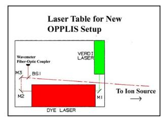
**Figure III.5**: Setup of the laser table in ion source room near OPPLIS. The laser table was completely contained within a small clean room with a clean-air filter. The dye laser beam was passed to OPPLIS through a small hole in the plastic surrounding the clean room.
