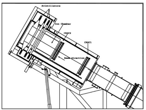
Figure I.10: A close up of the S800 focal plane detectors, taken from [23].
