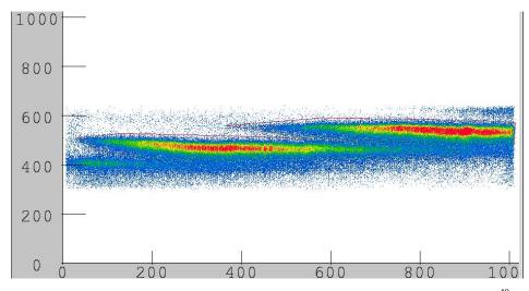
**Figure I.21**: TOF OBJE2 vs. CRDC1x spectrum showing mass ID of Sulfur events from the <sup>40</sup>S beam. <sup>39</sup>S events are shown by the red particle group on the left of the spectrum and <sup>38</sup>S events are shown by the red particle group on the right of the spectrum.
