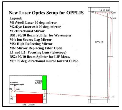
Figure III.8: Laser optics for new OPPLIS setup.
