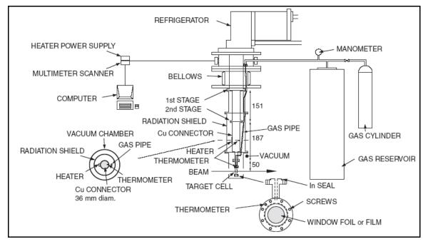
Figure I.7: Schematic view of the liquid hydrogen target taken from [18].
