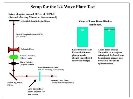
Figure C.1: <sup>1</sup>/<sub>4</sub> - wave plate test diagram
