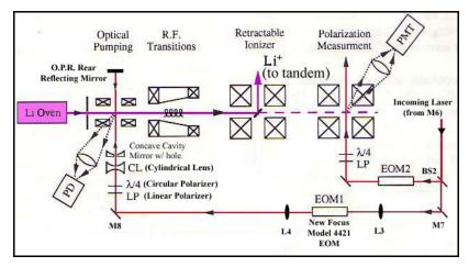
Figure III.7: Close-up of laser optics leading to optical pumping region in OPPLIS
