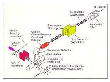
Figure III.4: Beam focusing elements of OPPLIS.
