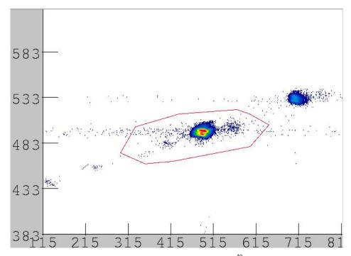
**Figure I.18**: *TOF XFPE2* vs. *TOF OBJE2* beam ID spectra for the <sup>40</sup>S elastic scattering run. Again, the events associated with the <sup>40</sup>S beam particles are centered in the spectrum (longer TOF) while the <sup>42</sup>Cl beam particles are to the right of the spectrum (shorter TOF).
