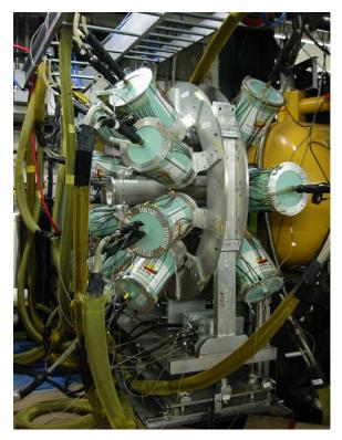
**Figure I.9**: Picture showing the Sega Array setup in front of Q1 and Q2 of the S800. Liquid deuterium target is not shown.
