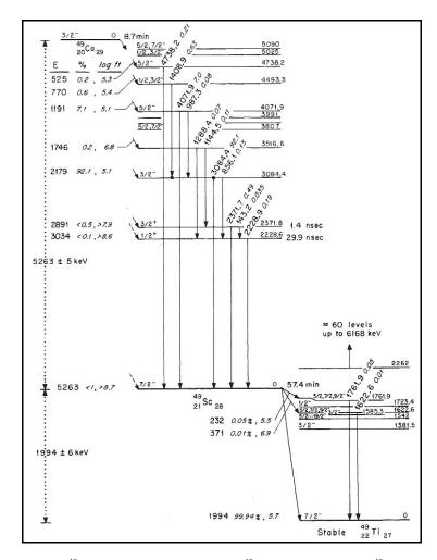
**Figure I.1**:  $\beta^-$ -decay of <sup>49</sup>Ca creating excited states in <sup>49</sup>Sc. Excited states in <sup>49</sup>Sc are observed via their characteristic gamma decays [5].
