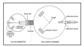
Figure III.10: 85cm scattering chamber setup for tests of OPPLIS.
