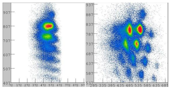
**Figures I.14a and I.14b**: Energy loss vs. TOF OBJE2 spectra before (left panel) and after (right panel) TOF correction. Note that the elements are separated into groups of isotopes in the right panel.
