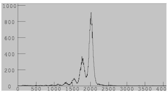
**Figure I.19**: 1D IC\_SUM energy loss spectrum gated on events associated with the <sup>40</sup>S beam. The energy loss of the sulfur peak is identified in the ion chamber with the beam elastic scattering run. The largest peak in the spectrum shows the reactions producing sulfur isotopes.
