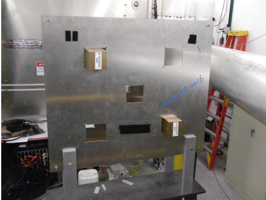
Figure 2.11: Brass shadowbars placed in one of four position configurations used during the experiment. One neutron wall is immediately behind the shadowbar mount. The outgoing beam pipe is seen on the right of the photo.
