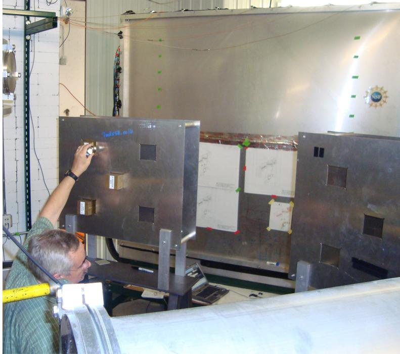
Figure 3.4: Dave Sanderson measured the shadowbar locations using a laser measurement system. The NW Array is seen behind the shadowbar mount.
