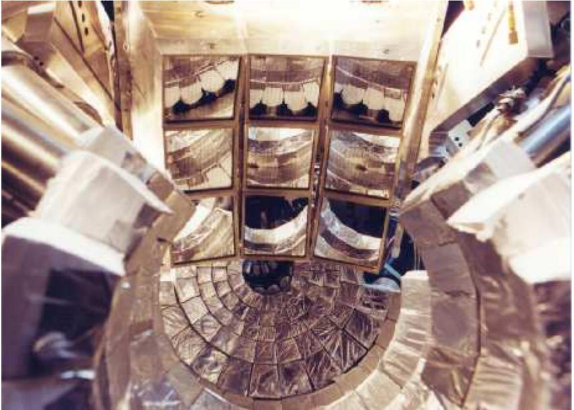
Figure 2.3: Miniball/Miniwall + LASSA detector setup viewed inside from the beam direction.
