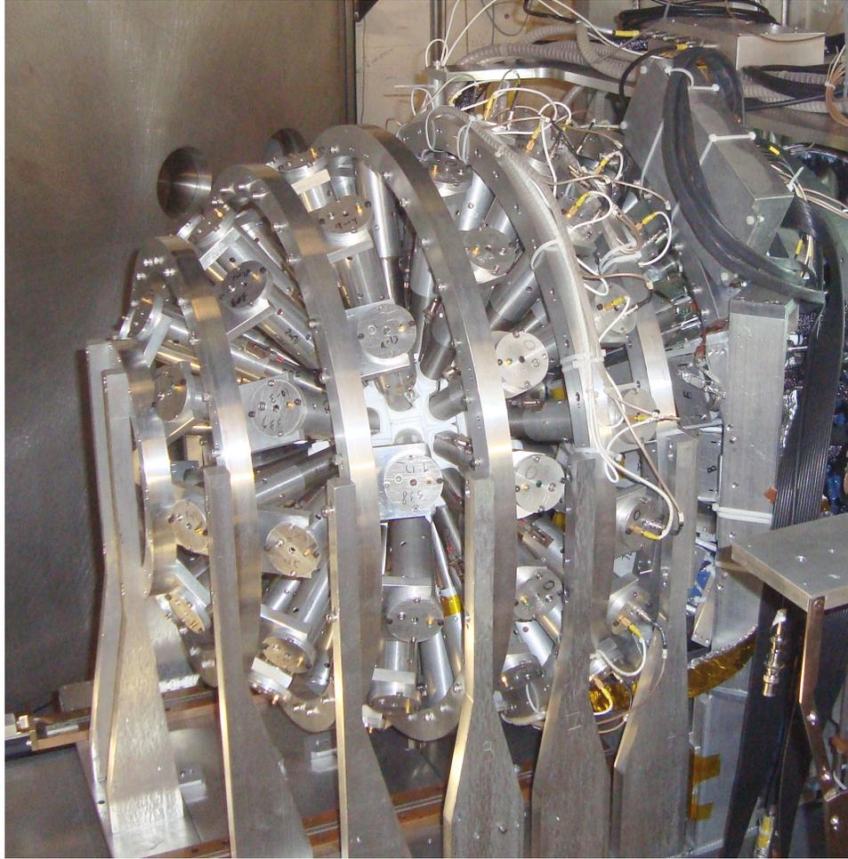
Figure 3.8 Fully assembled Miniball-Miniwall array, showing the backward rings. The beam is incident from the left, and the target is at the geometric center of the miniball.
