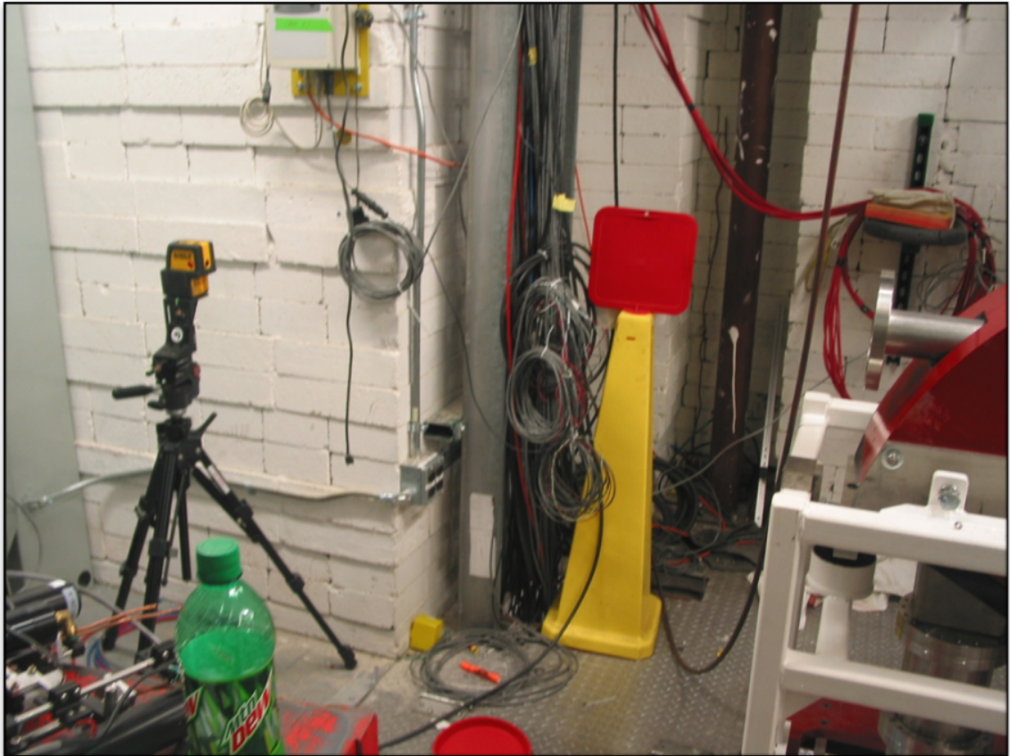
Figure 4.3: The laser was positioned behind the analyzing magnet, sending a laser beam back toward the selecting magnet
